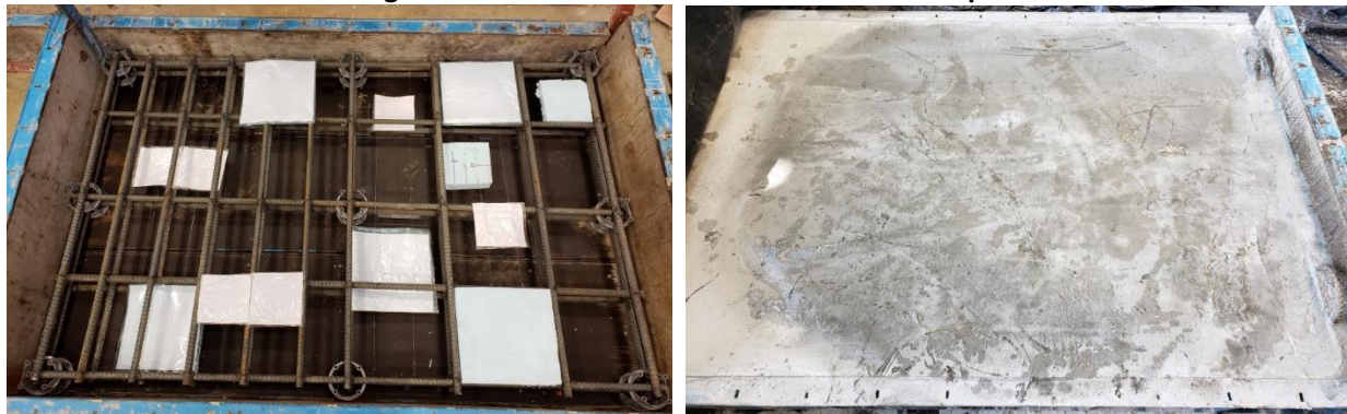
Figure 3-43: Pictures of the delamination sample before and after concrete pour.
