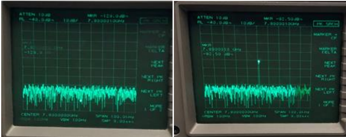
Noise floor of spectrum analyzer below -110 dBm
