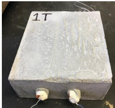
Figure 3-2: Sample with 1" cover, 55% W/C.
