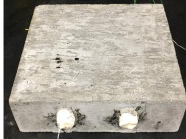
Figure 3-1: Original concrete block with embedded rebars.
