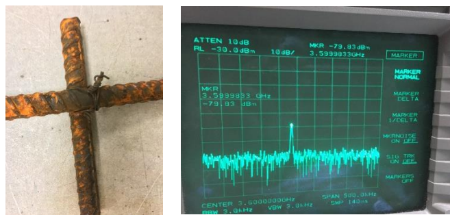
Figure 3-35: Configuration of rebars after 24-hours corrosion (left) and the measured 3 rd -order harmonic (right).
