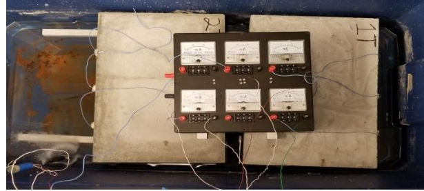
Figure 3-5: Corrosion salt bath setup with corrosion box centered on top.
