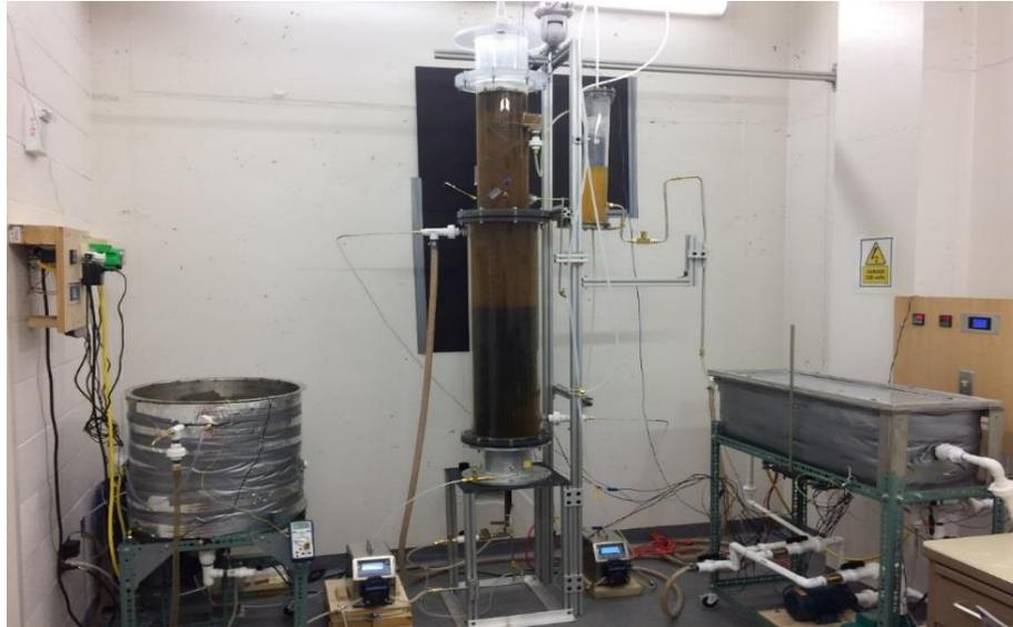
Figure 3. Two-Stages Expanded Granular Sludge Bed Reactor System
