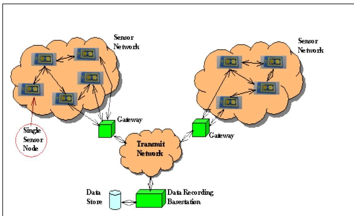
Figure 1.1. Typical structure of wireless sensor network
