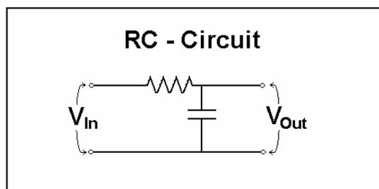
Fig. 3. Integrator circuit.
