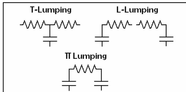
Fig. 2. Lump systems configurations.
