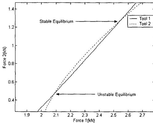
Fig. 7. Plot of Equation (17a) = 0 (solid line) and Equation (17b) = 0 (dotted line).  $m_1 = 1.5$  s,  $m_2 = 1.49$  s, and Controller Gains Given by Equation (15).
