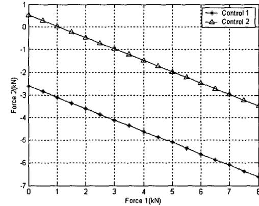
Fig. 9. Plot of Equation (21) = 0 for  $i = 1$  (stars) and  $i = 2$  (triangles) Illustrating Control Saturation Boundaries for the First and Second Tool, Respectively.  $m_1 = 1.5$  s,  $m_2 = 1.49$  s, and Controller Gains Given by Equation (15).
