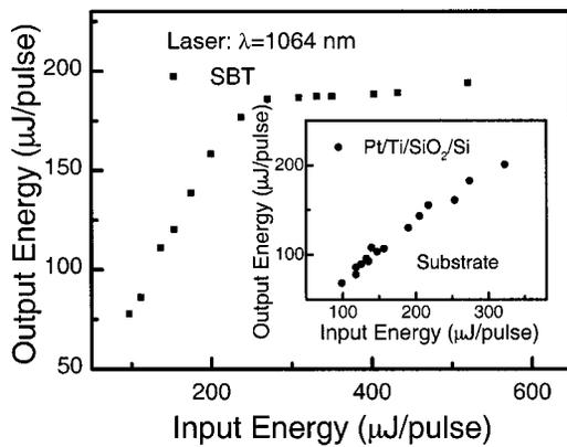
FIG. 1. Optical limiting of SBT ferroelectric thin film and the platinumized silicon substrate (inset) measured at 1.064 μm with 8 ns laser pulses.
