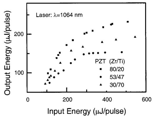
FIG. 2. Optical limiting of PZT ferroelectric thin films with varied Zr content ( $x=0.30, 0.53, \text{ and } 0.80$ ) at 1.064 μm with nanosecond laser pulses.
