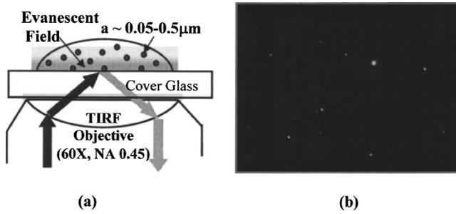
FIG. 1. (a) Operating principle of high-numerical-aperture (oil-immersion type) objective based TIRFM. The penetration depth  $z_p$  of the evanescent wave is 272 nm. (b) 100-nm-radius nanoparticles at the illumination conditions described in (a).
