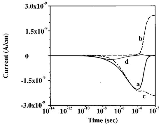
FIG. 5. Terminal drain current and its components: curves; a, is equal to  $I_d$ ; b, is equal to  $I_n$ ; c, is equal to  $I_p$ ; and d, is equal to  $I_{dis}$ . High density of trap states in Fig. 3, curve a is used. This figure can be compared to the corresponding crystalline silicon transistor of Fig. 1. Note that the drain current,  $I_d$ , is in the opposite flowing direction and that the displacement  $I_{dis}$  is always small.
