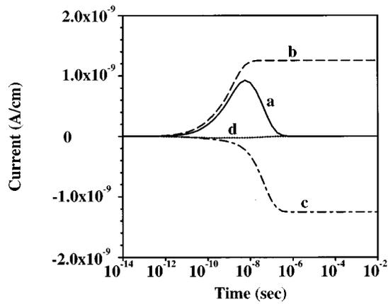
FIG. 1. Transient terminal drain current and its components: Curve a,  $I_d$ , total drain current, curve b,  $I_n$ , the electron component; curve c,  $I_p$ , the hole component, and curve d,  $I_{dis}$ , the displacement current component. The decompositions of  $I_d$  into  $I_n$ ,  $I_p$ , and  $I_{dis}$  are shown throughout the remaining figures.
