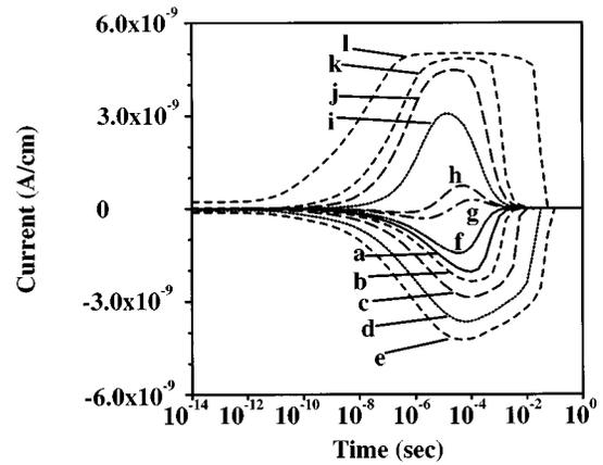
FIG. 12. Transient terminal drain current,  $I_d$ , as function of time. Each curve is for a different applied gate voltage: curves; a,  $V_G=0$ ; b,  $V_G=0.2$ ; c,  $V_G=1$ ; d,  $V_G=5$ ; e,  $V_G=15$ ; f,  $V_G=-0.1$ ; g,  $V_G=-0.18$ ; h,  $V_G=-0.2$ ; i,  $V_G=-0.3$ ; j,  $V_G=-0.5$ ; k,  $V_G=-1$ ; and l,  $V_G=-15$  V. Note that an interesting cross-over behavior occurs at  $V_G=-0.18$  V in curve g.
