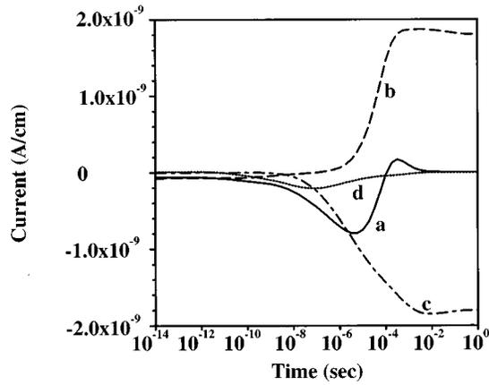
FIG. 8. (a) Terminal drain current,  $I_d$ , and its components: curves; a,  $I_d$ ; b,  $I_n$ ; c,  $I_p$ ; and d,  $I_{dis}$ . (b) Terminal source current,  $I_s$ , and its components: curves; a,  $I_s$ ; b,  $I_n$ ; c,  $I_p$ ; and d,  $I_{dis}$ . The medium density of trap states in Fig. 3, curve b is used. Note that the transient current exhibits an interesting cross-over behavior.
