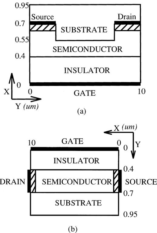
FIG. 2. Device geometries investigated: (a) shows a realistic  $U$ -shaped geometry of  $a$ -Si:H TFT with source and drain dopings indicated by the two shaded areas, (b) shows a rectangular geometry of  $a$ -Si:H TFT. In the computation  $l=10\ \mu\text{m}$  (channel length),  $\mu_n=20\ \text{cm}^2/\text{V}\cdot\text{s}$  and  $\mu_p=0.2\ \text{cm}^2/\text{V}\cdot\text{s}$  are used.
