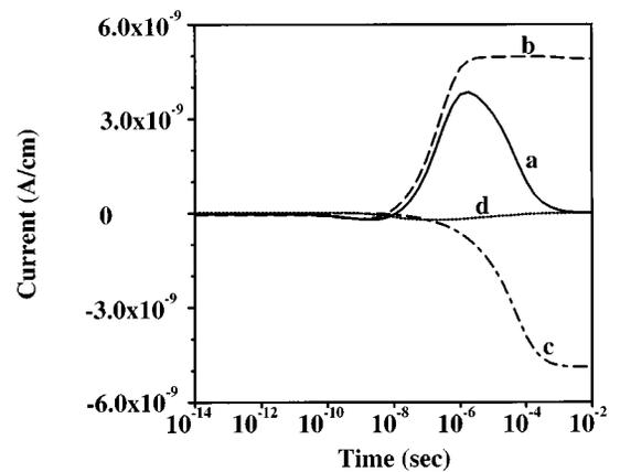
FIG. 7. Terminal drain current,  $I_d$ , and its components: curves; a,  $I_d$ ; b,  $I_n$ ; c,  $I_p$ ; and d,  $I_{dis}$ . The low density of trap states in Fig. 3, curve c is used. Note that the transient current peak is positive which is opposite to the sign in Fig. 5. In addition, the location of the transient peak is two orders of magnitude longer as compared to that of Fig. 1 of the crystalline case.
