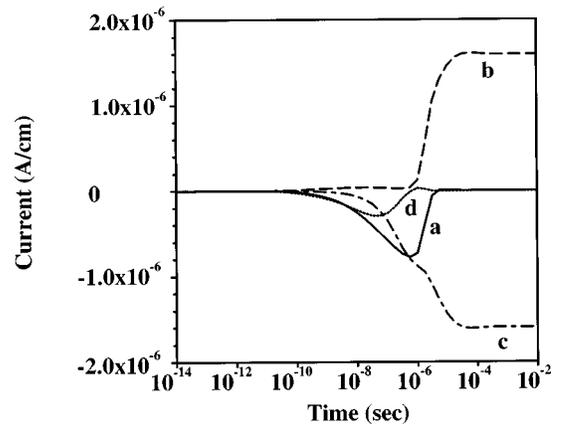
FIG. 6. Terminal drain current,  $I_d$ , and its components: a,  $I_d$ ; b,  $I_n$ ; c,  $I_p$ ; and d,  $I_{dis}$ . The high density of trap states in Fig. 3, curve a is used. Compared to Fig. 5, we note that when the illumination intensity is increased, the value of the transient current peak is larger and the location of the current peak is moved to the left of time scale because more electron-hole pairs are generated to fill the trap states.
