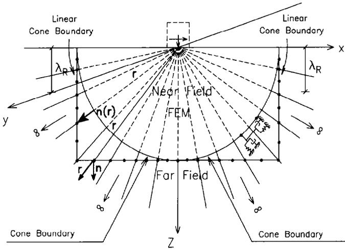
Fig.1. Transmitting boundaries for 3D FEM analysis. Plane view.
