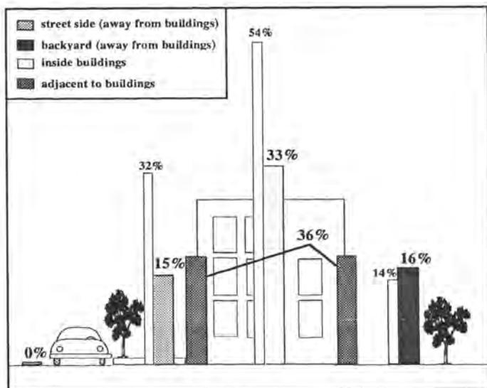
Fig 2. The location of the sand boils relative to the buildings, backyards and pavement in the Marina District.
