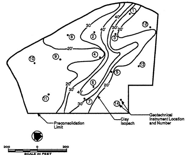
FIGURE 2. CLAY ISOPACH AND GEOTECHNICAL INSTRUMENT LOCATIONS
