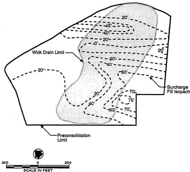
FIGURE 4. WICK DRAIN LIMIT AND SURCHARGE FILL ISOPACH
