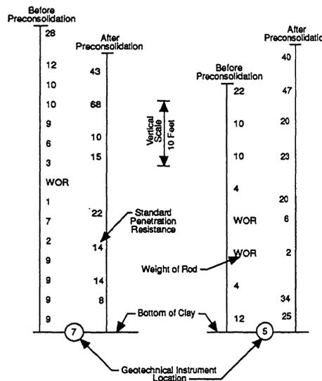
FIGURE 7. STANDARD PENETRATION RESISTANCE BEFORE AND AFTER PRECONSOLIDATION
