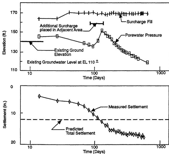
FIGURE 5. SETTLEMENT AND PIEZOMETER MEASUREMENTS FOR INSTRUMENT LOCATION 2
