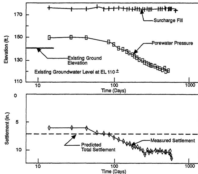
FIGURE 6. SETTLEMENT AND PIEZOMETER MEASUREMENTS FOR INSTRUMENT LOCATION 3
