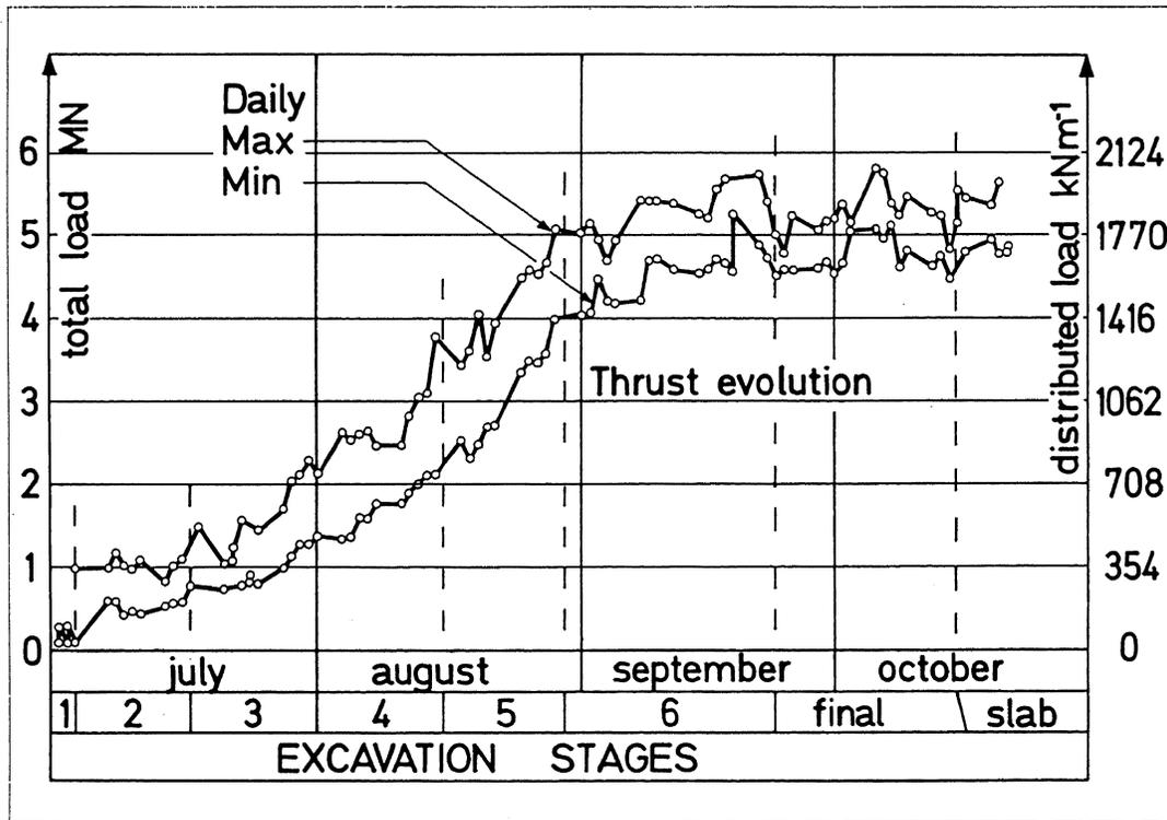
Fig. 5. Confederation Centre. Excavation#4. Thrust evolution.
