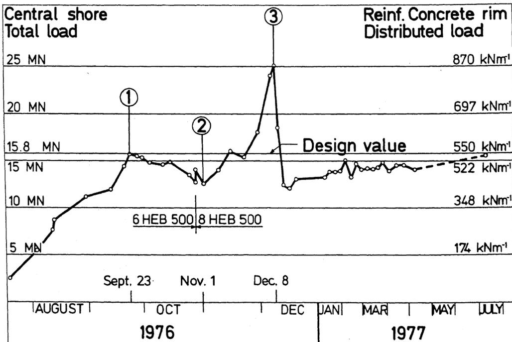
Fig. 10. Grand Casino. Thrust evolution on the central shore.
