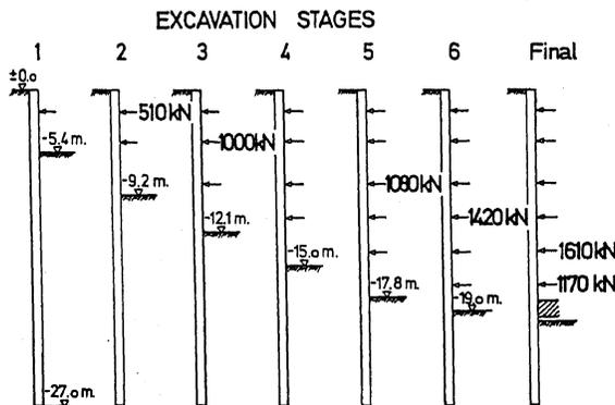
Fig. 6. Confederation Centre. Excavation#4. Excavation stages and maximum loads values.
