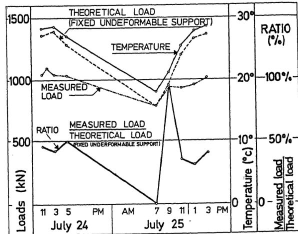
Fig. 7. Confederation Centre. Strut level Load variations with temperature increase. Extensometer readings.
