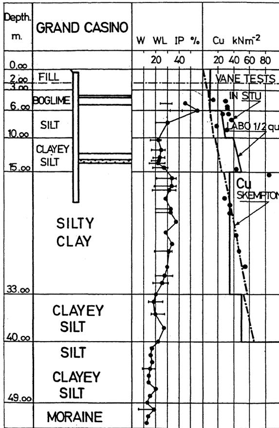
Fig. 8. Grand Casino. Geotechnical characteristics.
