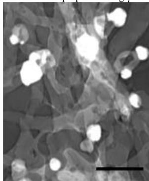
**Figure 1.** TEM of polyaniline/Ag composite nanoparticles. The Ag nanoparticles (bright spots) are attached to polyaniline fibers (medium brightness). The scale bar represents 50 nm.
