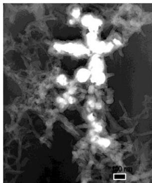
**Figure 2.** TEM of polyaniline/Au composite nanoparticles. The Au nanoparticles (bright spots) are attached to polyaniline fibers (medium brightness). The scale bar represents 100 nm.
