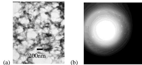
**Figure 4.** (a) TEM image of PEDOT/CdS nanocomposite. (b) SAED image showing the reflection from (101), (110) and (103) planes of CdS.
