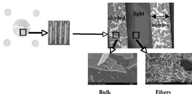
**Figure 3.** (L) Optical microscopic image of the patterning employed to produce bulk/nanofiber polyaniline thin films. (R) Optical and SEM images of patterned polyaniline thin films. The darker, uniform region was illuminated, and consisted of nanofibers. The shaded areas consisted of bulk polyaniline.
