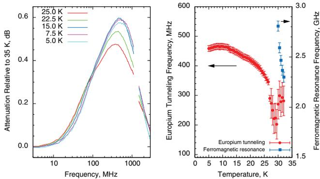
FIG. 3 (color). The microwave attenuation in  $\text{Eu}_8\text{Ga}_{16}\text{Ge}_{30}$  at different temperatures, left. A resonant cavity in the instrument prevents measurements at  $\sim 1300$  MHz. The frequency of both the maximum in power absorption attributed to the Eu tunneling, in red, and the ferromagnetic resonance, observed near  $T_C$ , in blue, are shown on the right.
