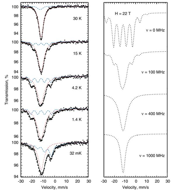
FIG. 2 (color). The Mössbauer spectra of  $\text{Eu}_8\text{Ga}_{16}\text{Ge}_{30}$  obtained at the indicated temperatures, left. The solid black line is the total fit obtained from the sum of the magnetic subspectrum assigned to Eu(A), the blue curve, and the relaxation subspectrum assigned to Eu(B) the red curve. The calculated spectra for divalent Eu with a 22 T hyperfine field that is randomly fluctuating at the indicated frequencies, right.
