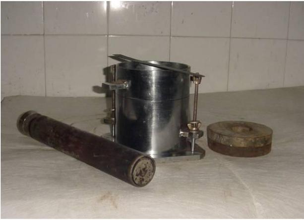
Fig. 3. Standard CBR Mould set-up
