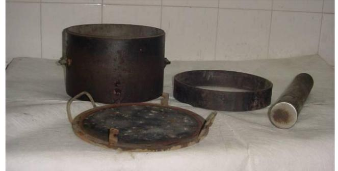
Fig. 4. Modified CBR Mould
