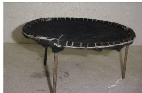
Fig. 5. Circular ring holding the geotextile in position
