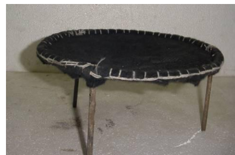
Fig. 5. Circular ring holding the geotextile in position
