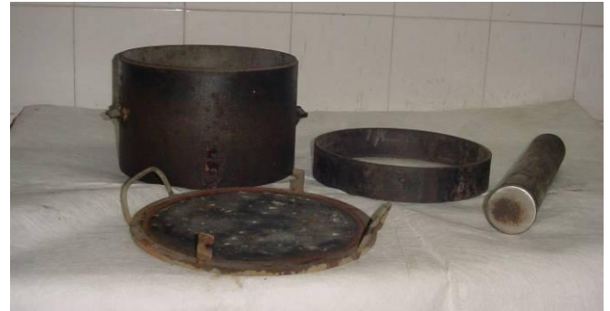
Fig. 4. Modified CBR Mould
