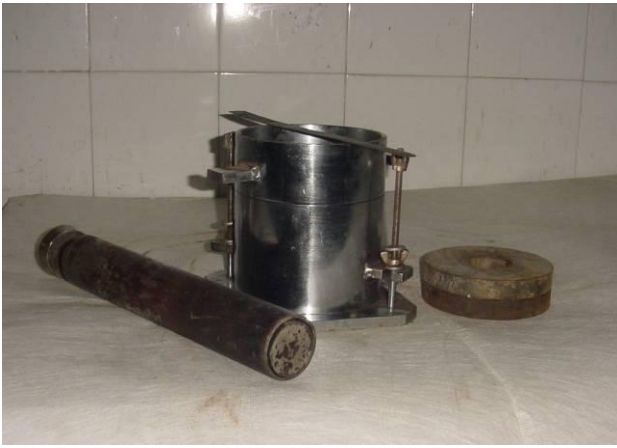
Fig. 3. Standard CBR Mould set-up
