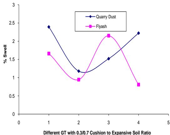
Fig. 10. Comparison between Different geotextiles in Locked condition
