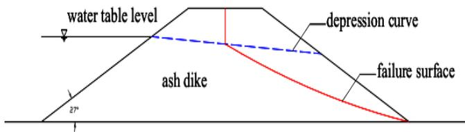
Fig. 5. Structure of ash dike.
