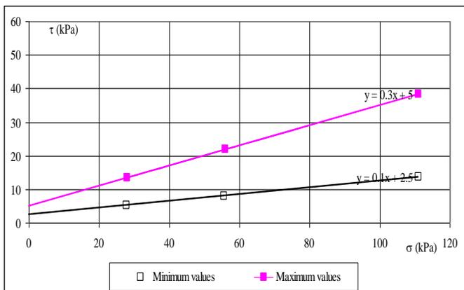
Fig. 3. Shear strength diagram for ash.
