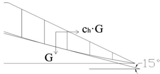
Fig. 8. Typical seismic forces acting on the slip surface.
