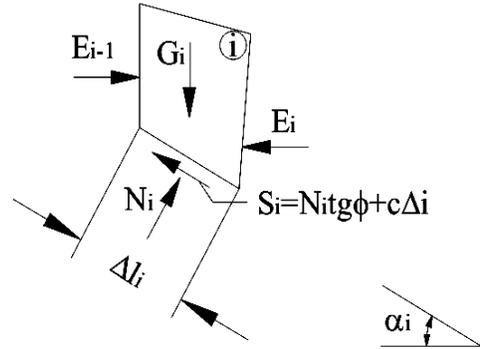
Fig. 10. General calculation scheme for STAB-1 (after Athanasiu et al., 1983).
