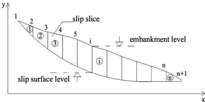
Fig. 9. General calculation scheme used by STAB-1 (after Athanasiu et al., 1983).
