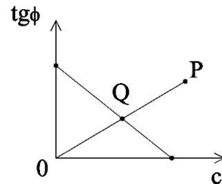
Fig. 11. Shear parameters envelope for limit equilibrium (after Athanasiu et al., 1983).
