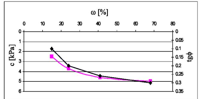
Fig. 12. Ash humidity versus shear strength parameters.
