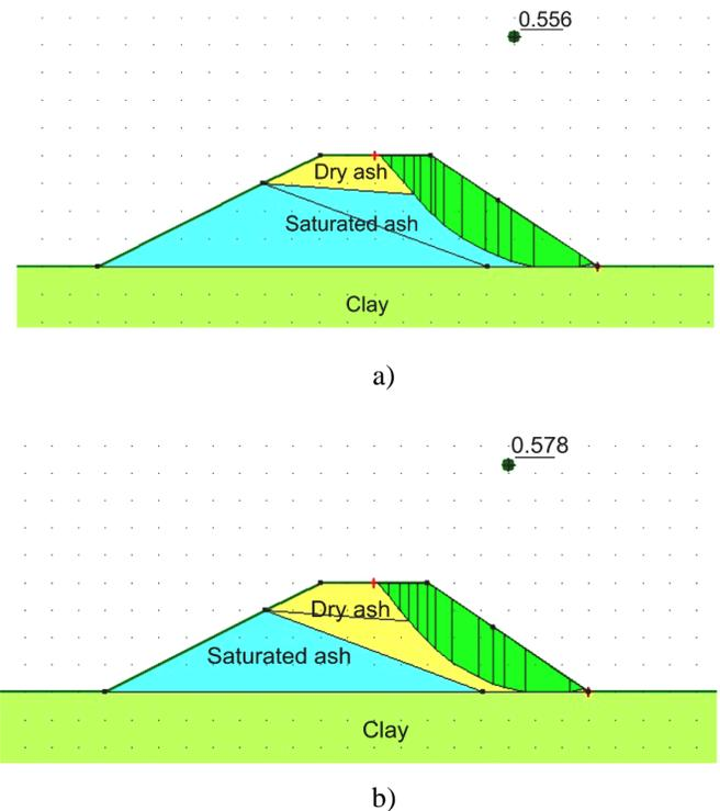
Fig. 6. Detail of slope analysis modeling for  $c = 2.5 \text{ kPa}$  and  $\text{tg } \phi = 0.1$  – a) without drainage system; b) with drainage system.
