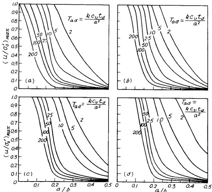
Fig. 6 Relationship between Max. Pore Pressure Ratio and Drain System Parameters
