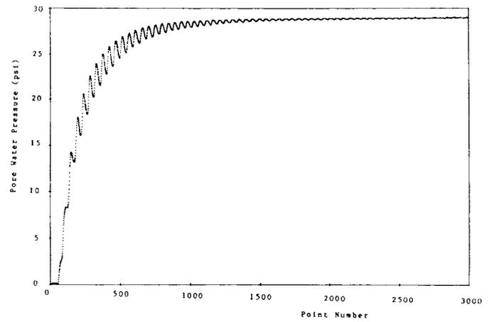
Figure 2. Pore Pressure Increase Leading to Soil Liquefaction
