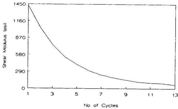
Figure 4. Shear Modulus Variation per Cycle before Liquefaction
