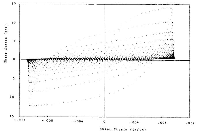
Figure 3. Characteristic Hysteresis Loops During a Liquefaction Test
