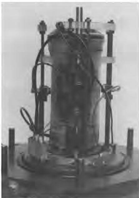
Fig. 3 Triaxial Apparatus
