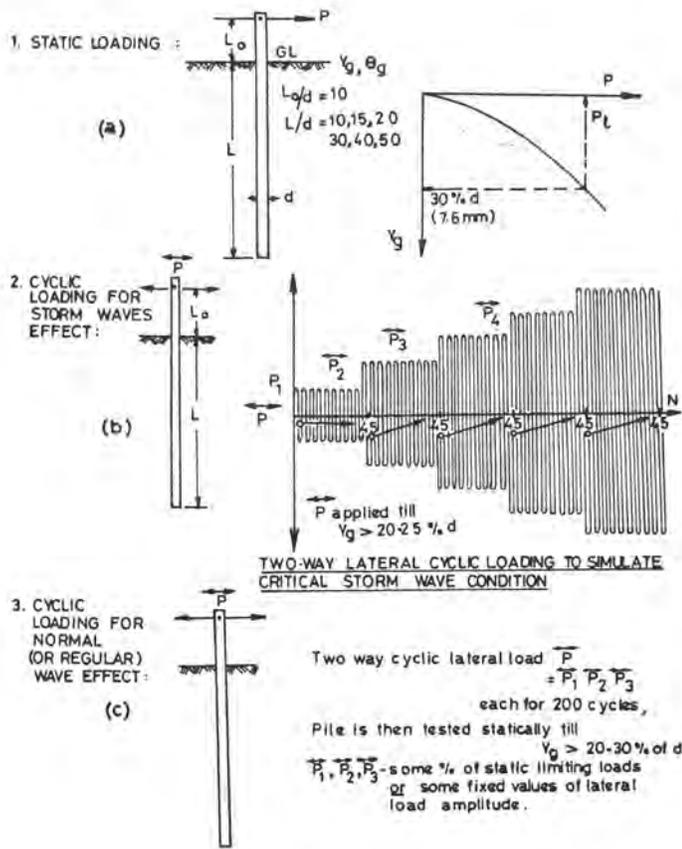
Figure 1. Idealised scheme of lateral loading on pile
