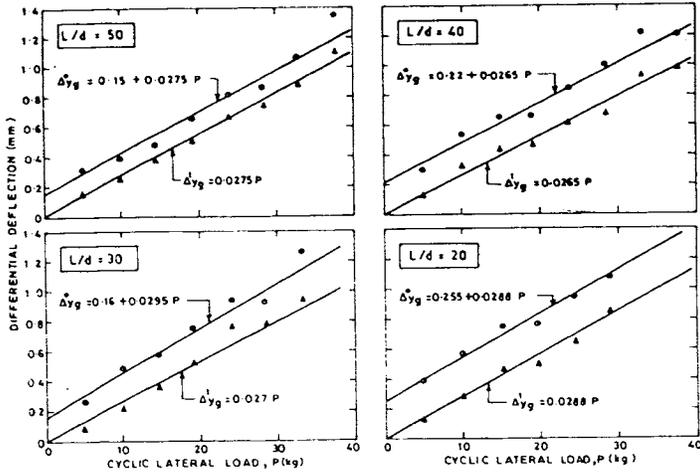
Figure 5. Differential deflections during CYS loading stages
