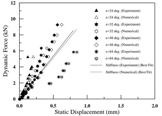
Fig. 8 Force vs. Static amplitude plot for Site-I
