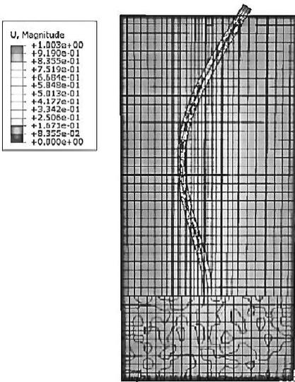
Fig. 6. Mode 4 of soil-pile system
