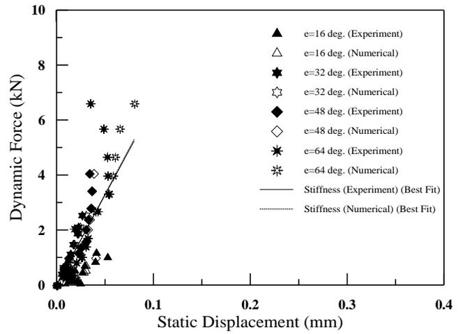
Fig. 9 Force vs. Static amplitude plot for Site-II
