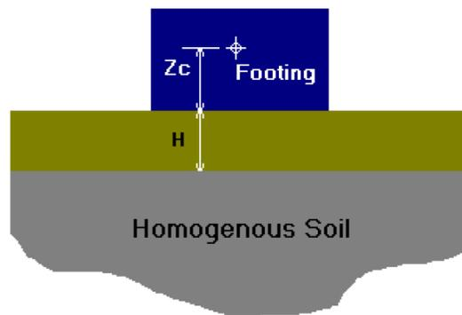
Fig. 10 Rigid footing resting on composite strata
