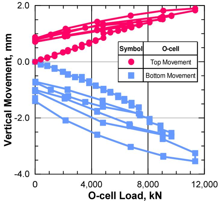
Fig. 4. Typical O-cell Load Displacement Curve, from O4
