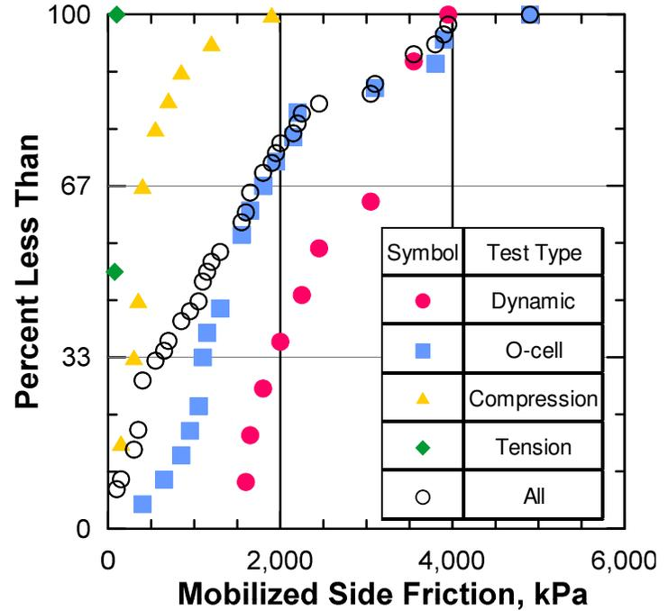
Fig 7. Cumulative Distribution of Mobilized Side Friction values by Test Type
