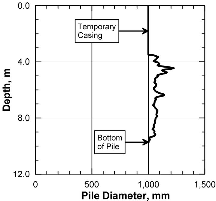
Fig. 9. Example of Caliper Logging Results, from O6
