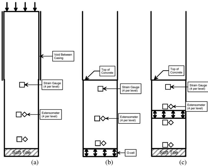
Fig. 1. Cross-Sections of Typical Preliminary Load Test Setups (a) Jack and Reaction-Frame with soft-toe, (b) O-cell at Base of Pile, and (c) O-cell at mid-point of shaft with soft-toe.
