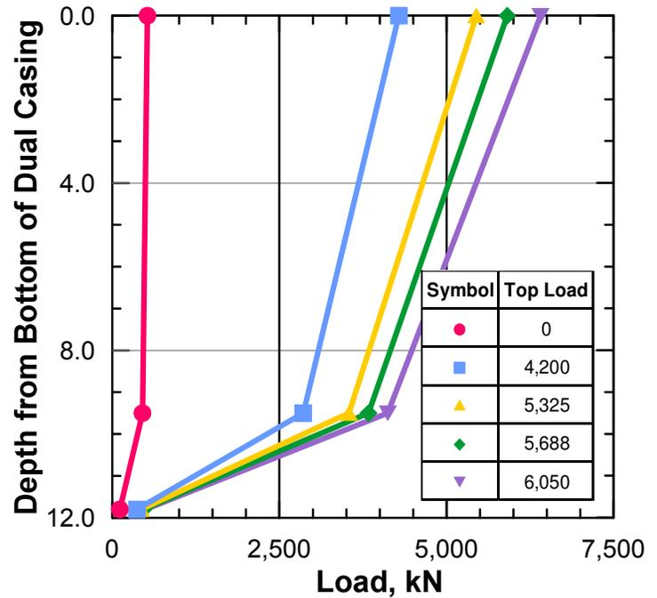
Fig. 3. Side Friction Load Distribution, from PC3
