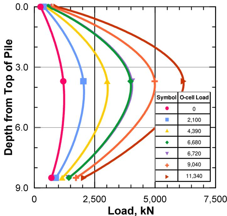
Fig. 5. Typical Side Shear Distribution, from O4
