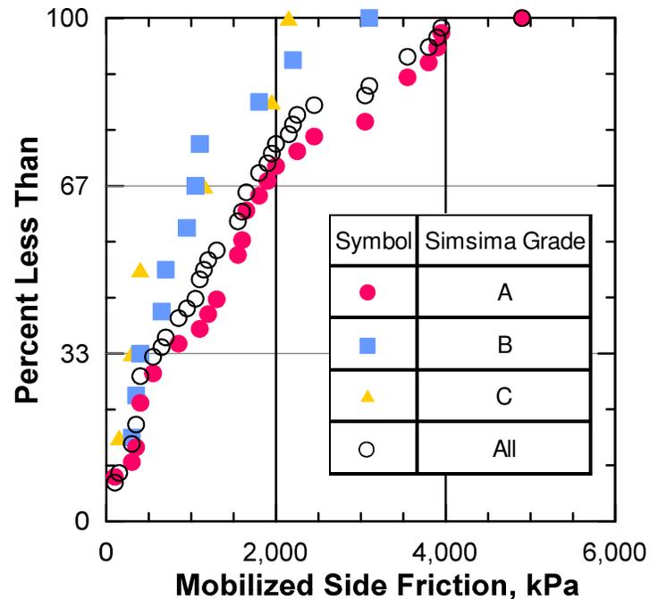
Fig 8. Cumulative Distribution of Mobilized Side Friction value by Grade of Simsima Limestone
