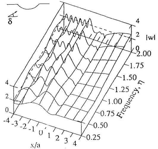
Figure 5. Shallow Semi-Cylindrical Canyon, Incident SH-Wave,  $h/a=0.5$ ,  $\delta=30^\circ$
