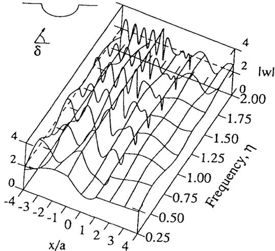
Figure 6. Shallow Semi-Elliptical Canyon, Incident SH-Wave,  $D/W=0.35$ ,  $\delta=60^\circ$
