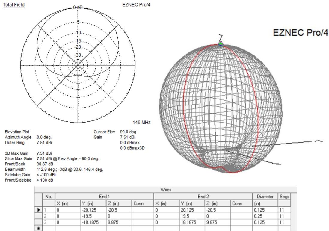
Figure 5. Three-element Yagi-Uda antenna with cardioid pattern.
