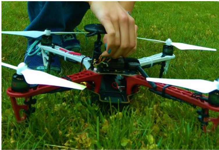
Figure 1. Model F450 Flame Wheel Quadcopter by DJI.
