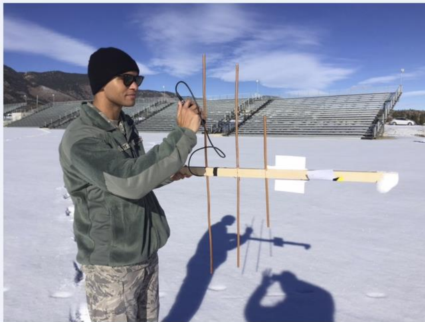
Figure 2. Transmitter Hunt with Directional Antenna in Two-Meter Band [1].
