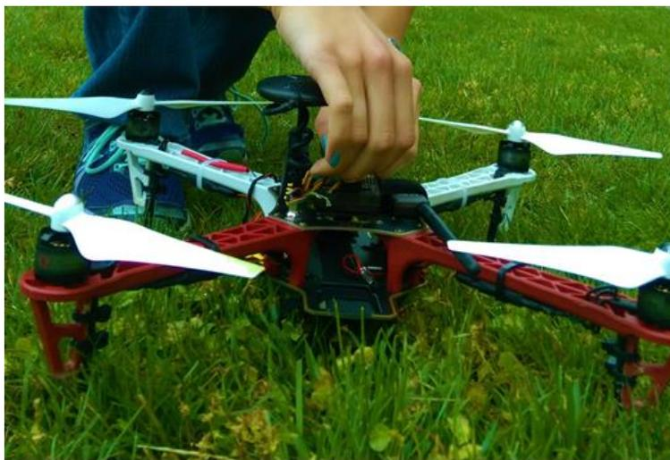
Figure 1. Model F450 Flame Wheel Quadcopter by DJI.
