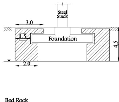
Fig. 4. Concrete bracket section
