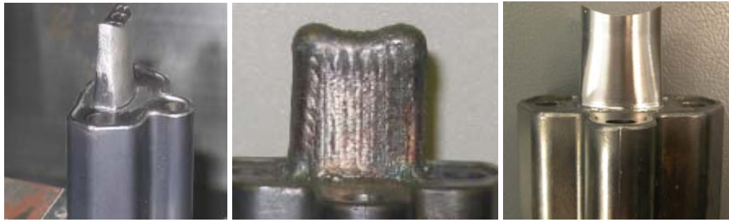
Figure 11 Die core repaired via surface patching (a) Before repairing (b) After deposition (c) After surface machining.
