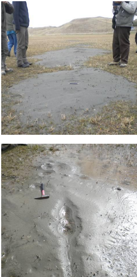
Fig. 6. Sand boils observed after the M_w 7.2 Van earthquake in the Karasu River floodplain near Topaktas village
