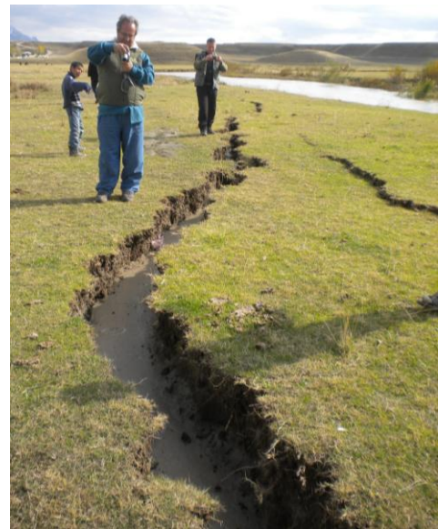
Fig. 7. Lateral spreading cracks observed after the M_w 7.2 Van earthquake in the Karasu River floodplain
