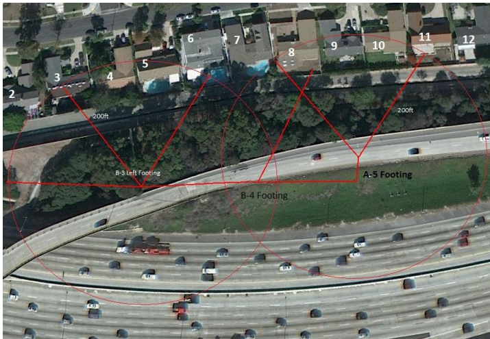
Fig. 1. Buildings within the 200ft of the pile driving
