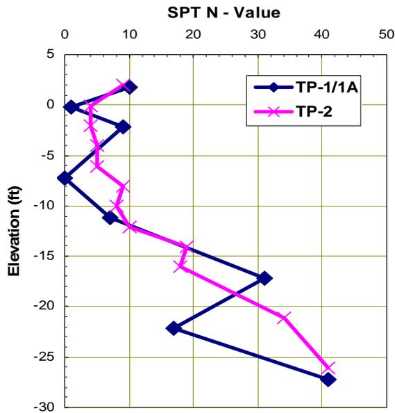
Fig 7. Subsurface Condition at Test Columns
