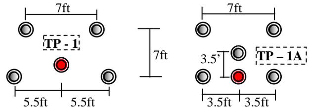
Fig 9. Test/Production Columns Layout
