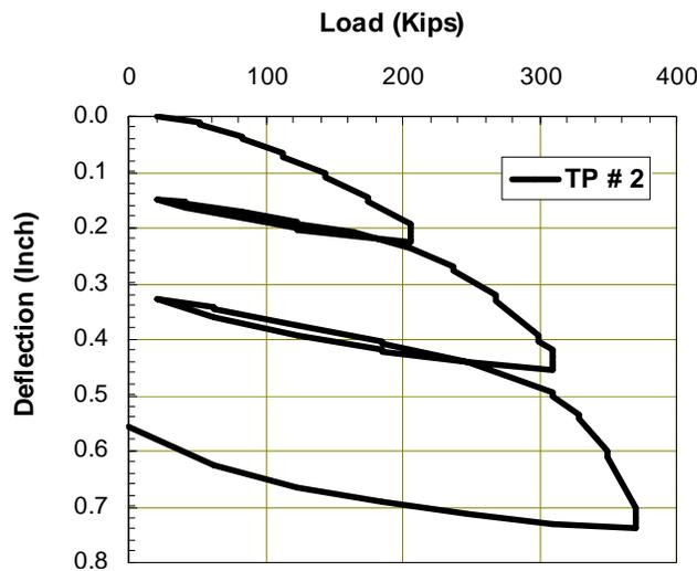
Fig 6. North Approach Test Column Result
