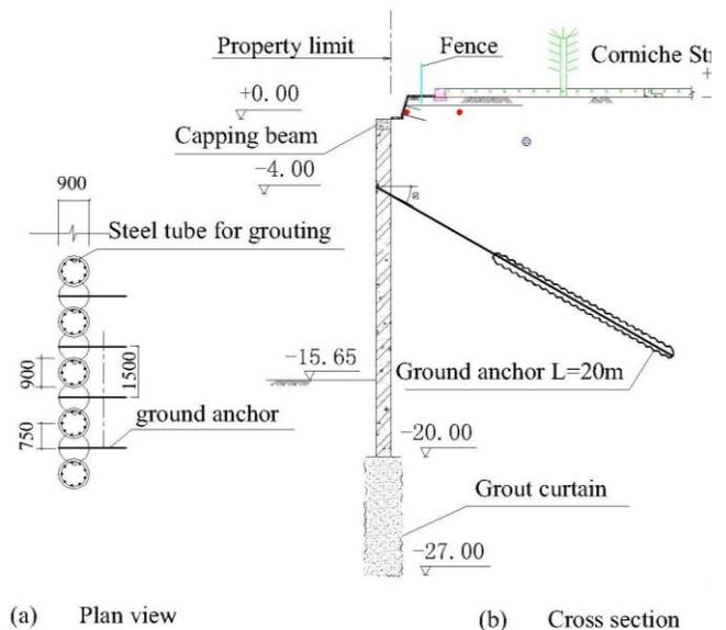
Fig. 1. Anchored secant pile wall with toe grouting
