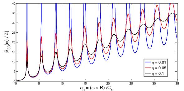
Fig. 3. Normalized dynamic stiffness per unit length of an infinite cylinder due to dynamic vertical load in the axial direction for different values of the loss factor, when  $E = 9411 \times 10^3$  and  $\nu = 0.495$ .
