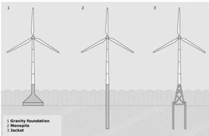
Fig. 1. Different types of offshore wind foundation.
