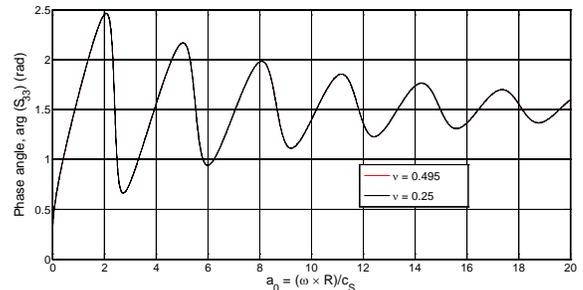
Fig. 8. Phase angle of an infinite hollow cylinder due to dynamic vertical load in the axial direction for different values of the Poisson's ratio  $\nu = 0.25$  and  $\nu = 0.495$  when  $E = 9411 \times 10^3 \text{ N/m}^2$  and the loss factor  $\eta = 0.1$ .
