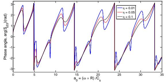
Fig. 12. Phase angle of an infinite solid cylinder due to dynamic vertical load in the axial direction for different values of the loss factor when the Young's modulus  $E = 9411 \times 10^3 \text{ N/m}^2$  and  $\nu = 0.495$ .
