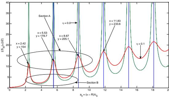
Fig. 9. Normalized dynamic stiffness versus different values of load's frequencies by having different values of loss factor  $\eta = 0.0$  and  $\eta = 0.1$  when  $\nu = 0.495$  and  $E = 9411 \times 10^3 \text{ N/m}^2$ .
