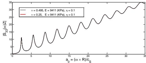
Fig. 5. Normalized dynamic stiffness per unit length of an infinite hollow cylinder due to dynamic vertical load in the axial direction for different values of the Poisson's ratio  $\nu = 0.25, \nu = 0.495$  when loss factor  $\eta = 0.1$  and  $E = 9411 \times 10^3 \text{ N/m}^2$
