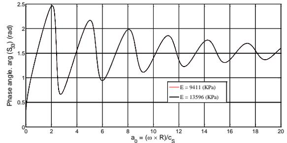
Fig. 7. Phase angle of an infinite hollow cylinder due to dynamic vertical load in the axial direction for different values of the Young's modulus  $E = 9411 \times 10^3 \text{ N/m}^2$  and  $E = 13596 \times 10^3 \text{ N/m}^2$  when loss factor  $\eta = 0.1$  and  $\nu = 0.495$ .
