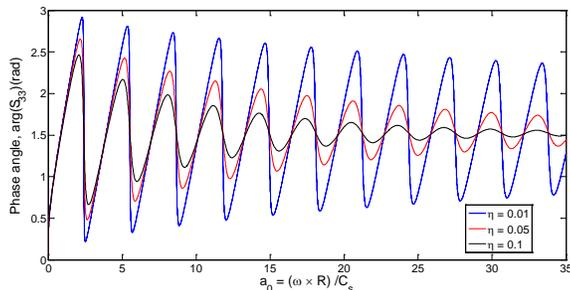
Fig. 6. Phase angle of an infinite hollow cylinder due to dynamic vertical load in the axial direction for different values of the loss factor when the Young's modulus  $E = 9411 \times 10^3 \text{ N/m}^2$  and  $\nu = 0.495$ .
