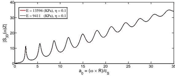
Fig. 4. Normalized dynamic stiffness per unit length of an infinite hollow cylinder due to dynamic vertical load in the axial direction for different values of the Young's modulus  $E = 9411 \times 10^3$ ,  $E = 13596 \times 10^3$  when loss factor  $\eta = 0.1$  and  $\nu = 0.495$ .
