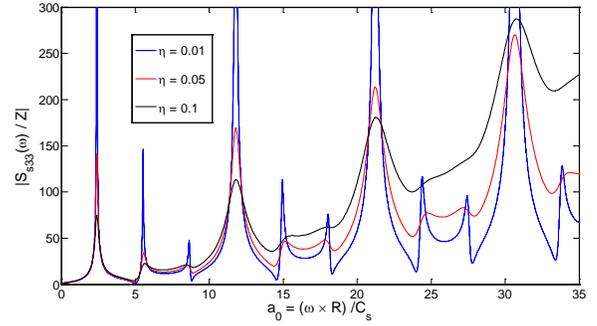
Fig. 11. Non-dimensional dynamic stiffness per unit length of an infinite cylinder due to dynamic vertical load in the axial direction for different values of the loss factor, when  $E = 9411 \times 10^3$  and  $\nu = 0.495$ .
