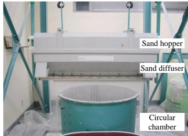
Fig. 4. Soil sample forming with sand diffuser
