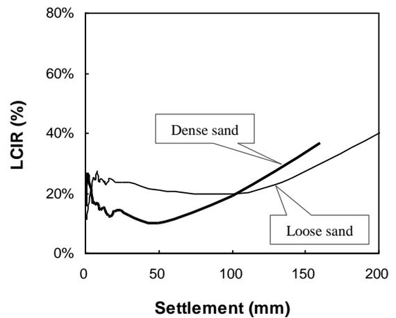
Fig. 10. Load capacity increase ratio in piled raft
