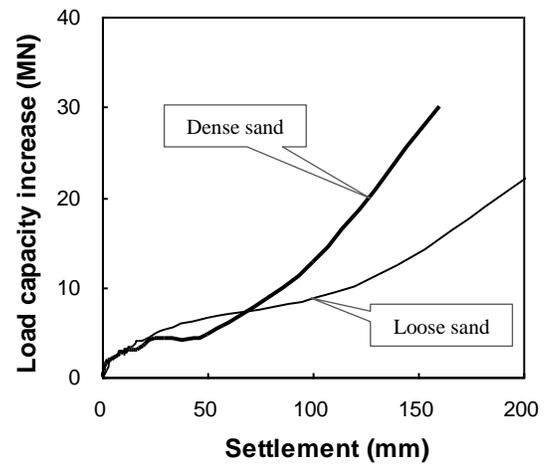
Fig. 9. Load capacity increase in piled raft
