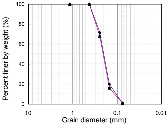
Fig. 5. Grain-size distribution of the test sands.
