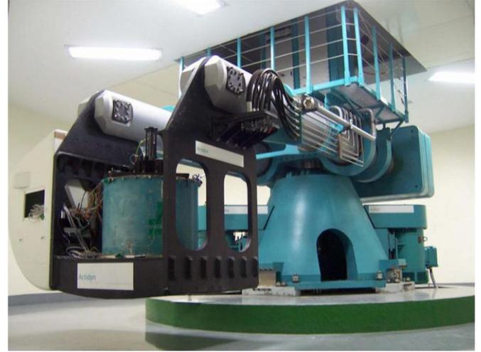
Fig. 3. Centrifuge testing system
