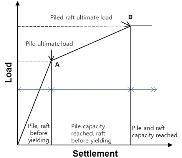
Fig. 2. Simplified contact piled raft load-settlement curve.
