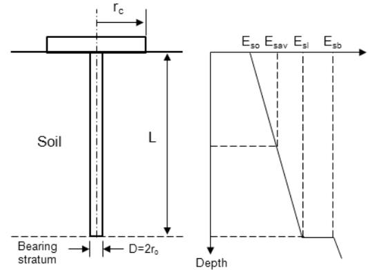
Fig. 1. Simplified representation of piledraft unit.
