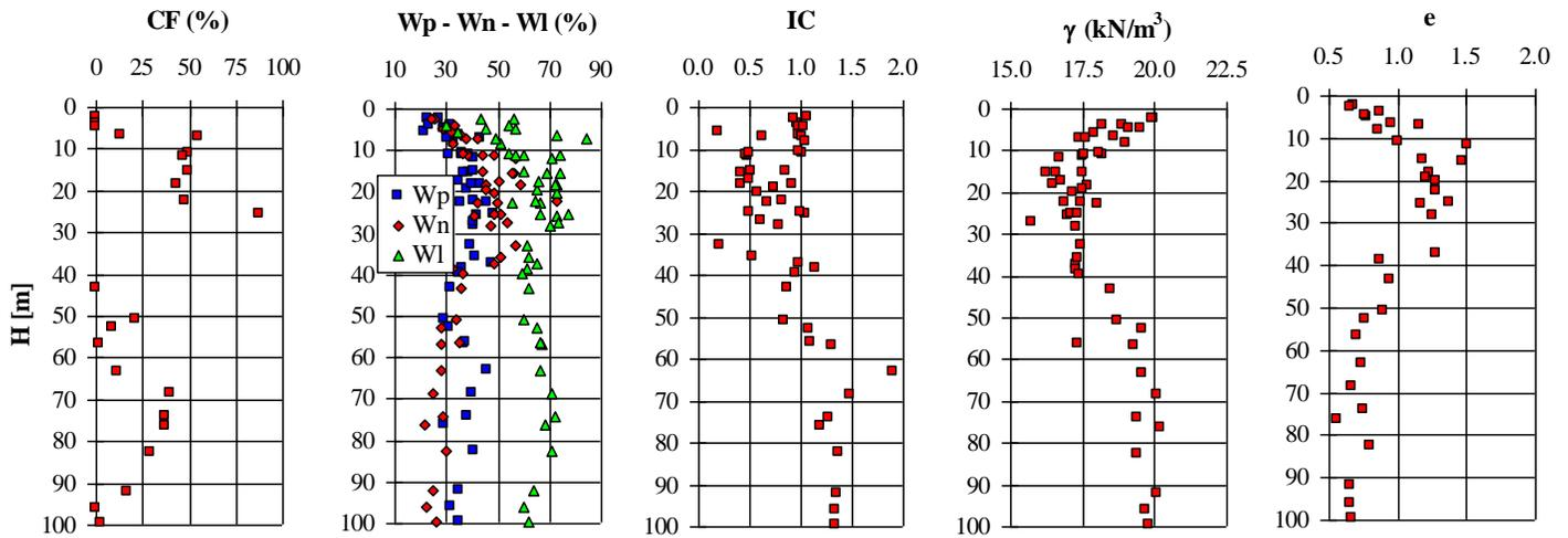
Fig. 2. Typical range of index properties of the clayey soils at the site of Industrial area of Catania STM-M6 (Italy).
