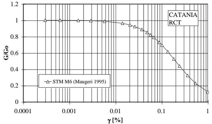
Fig. 7.  $G/G_o$ - $\gamma$  curves from RCT tests.
