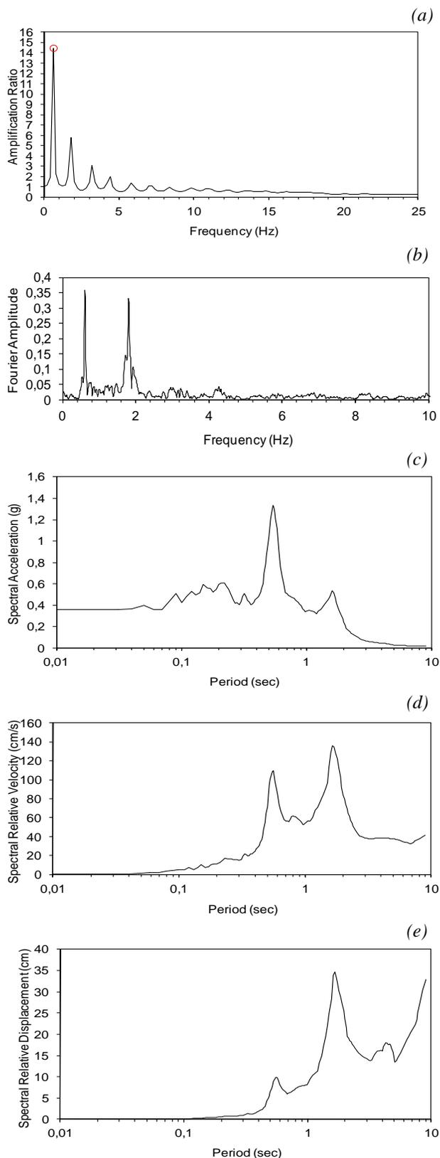
Figure 14. Site Response analysis results for the deterministic approach using the D-H soil profile. a) Amplification Ratio; b) Fourier amplitude; c) Spectral Acceleration; d) spectral velocity; e) spectral relative displacement.
