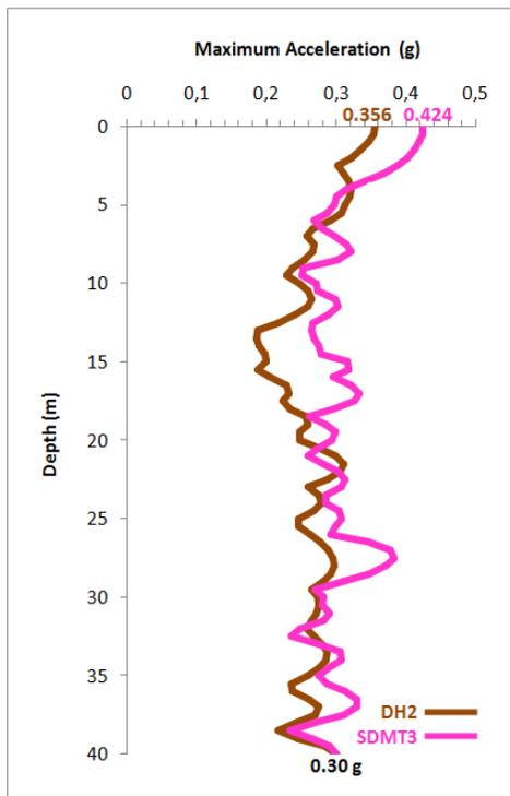
Fig. 12. Maximum accelerations with depth obtained from the response analyses for D-H and SDMT Vs profiles, using the Sortino input accelerogram scaled to 0.3g (deterministic approach).
