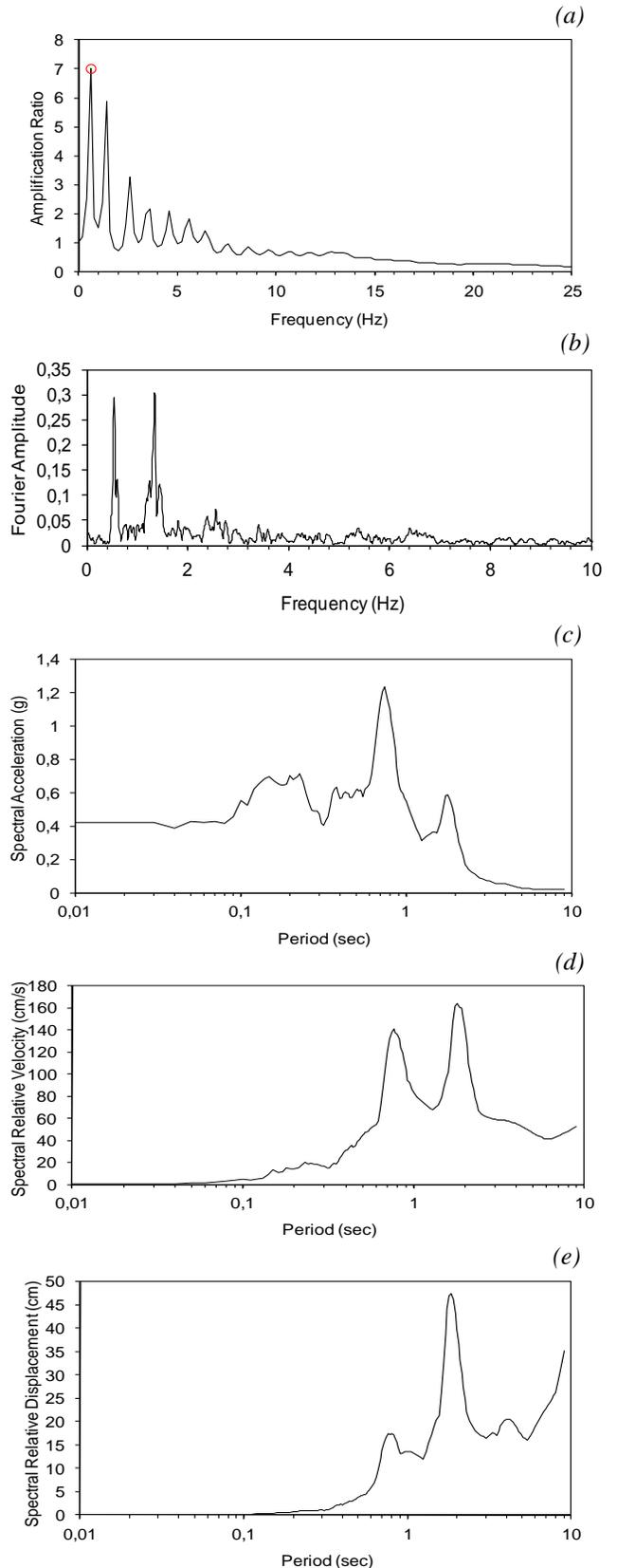
Figure 13. Site Response analysis results for the deterministic approach using the SDMT soil profile. a) Amplification Ratio; b) Fourier amplitude; c) Spectral Acceleration; d) spectral velocity; e) spectral relative displacement.
