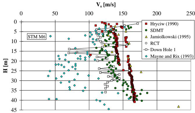
Fig. 9.  $V_s$  from laboratory and in situ tests.
