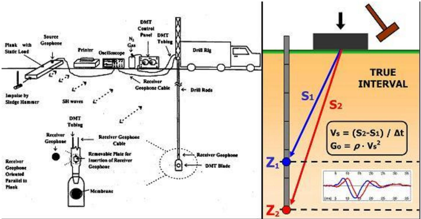
Fig. 4. The Seismic Dilatometer Marchetti Test (SDMT), resulting from the combination of the DMT blade with a modulus measuring the shear wave velocity  $V_s$ .
