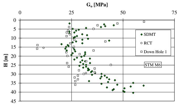
Fig. 6.  $G_o$  from laboratory and in situ tests.
