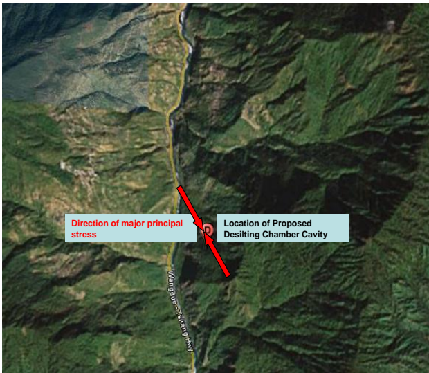
Fig. 9. Orientation of stress vis – a – vis Structural lineament and the river
