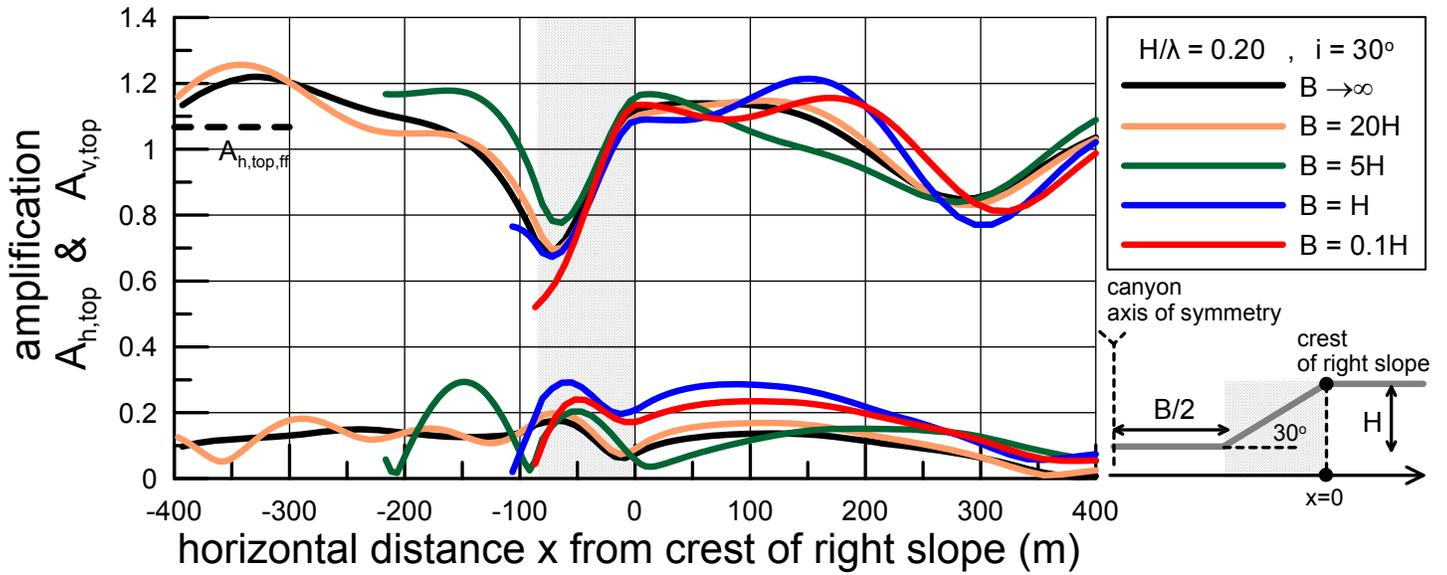
Fig. 3 Spatial variability of topographic aggravation factors  $A_{h,top}$  and  $A_{v,top}$  in the vicinity of symmetric trapezoidal canyons with slope inclination  $i=30^\circ$ , normalized height  $H/\lambda=0.20$  and various widths  $B = 0.1H, H, 5H, 20H$  and  $B \rightarrow \infty$ . Results are shown from the axis of symmetry of the canyon up to  $x=8H=400\text{m}$  behind the crest of the right slope.
