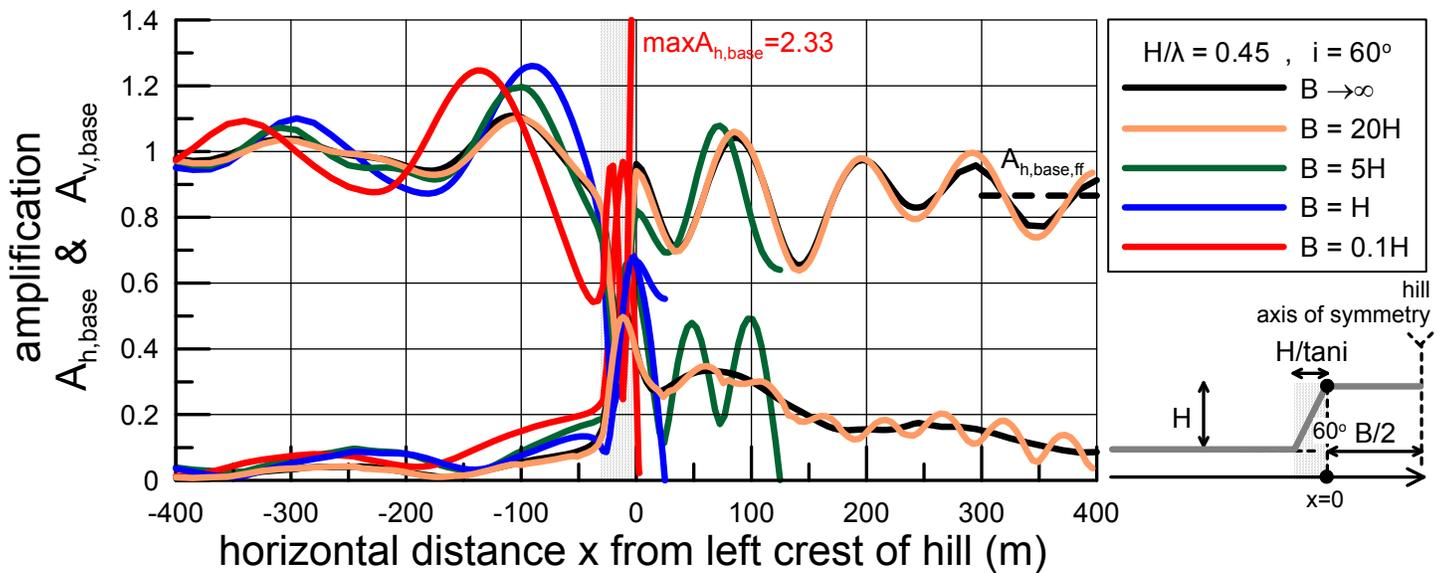
Fig. 14 Spatial variability of topographic aggravation factors  $A_{h,base}$  and  $A_{v,base}$  in the vicinity of symmetric trapezoidal hills with slope inclination  $i=60^\circ$ , normalized height  $H/\lambda=0.45$  and various widths  $B = 0.1H, H, 5H, 20H$  and  $B \rightarrow \infty$ . Results are shown from  $x=-8H=-400m$  in front of the toe of the left slope and reach the axis of symmetry of the hill.
