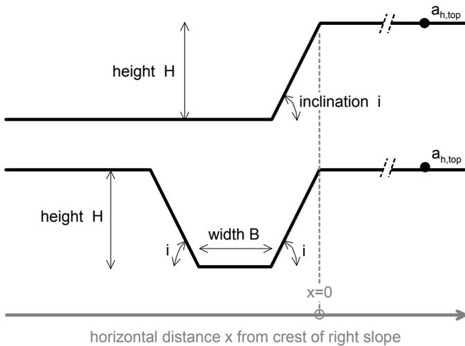
Fig. 1. Schematic illustration of 2D canyon with (inclination  $i$ , height  $H$ ) and respective 2D trapezoidal symmetrical hill of width  $B$ ; location of  $a_{h,base}$  used in the estimation of topographic aggravation
