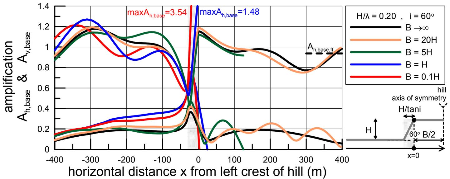
Fig. 13 Spatial variability of topographic aggravation factors  $A_{h,base}$  and  $A_{v,base}$  in the vicinity of symmetric trapezoidal hills with slope inclination  $i=60^\circ$ , normalized height  $H/\lambda=0.20$  and various widths  $B = 0.1H, H, 5H, 20H$  and  $B \rightarrow \infty$ . Results are shown from  $x=-8H=-400m$  in front of the toe of the left slope and reach the axis of symmetry of the hill.
