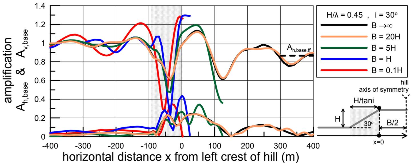
Fig. 10 Spatial variability of topographic aggravation factors  $A_{h,base}$  and  $A_{v,base}$  in the vicinity of symmetric trapezoidal hills with slope inclination  $i=30^\circ$ , normalized height  $H/\lambda=0.45$  and various widths  $B = 0.1H, H, 5H, 20H$  and  $B \rightarrow \infty$ . Results are shown from  $x=-8H=-400$ m in front of the toe of the left slope and reach the axis of symmetry of the hill.
