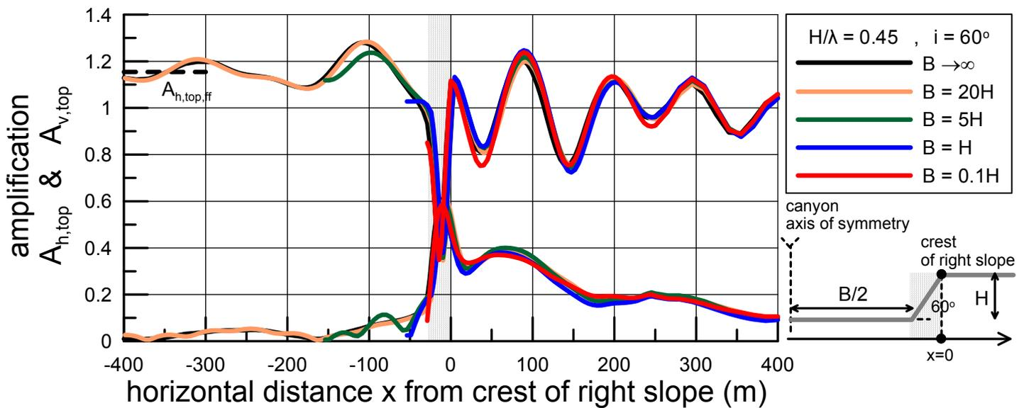
Fig. 8 Spatial variability of topographic aggravation factors  $A_{h,top}$  and  $A_{v,top}$  in the vicinity of symmetric trapezoidal canyons with slope inclination  $i=60^\circ$ , normalized height  $H/\lambda=0.45$  and various widths  $B = 0.1H, H, 5H, 20H$  and  $B \rightarrow \infty$ . Results are shown from the axis of symmetry of the canyon up to  $x=8H=400\text{m}$  behind the crest of the right slope.
