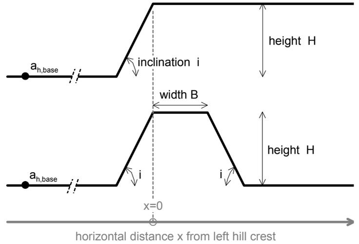
Fig. 2. Schematic illustration of 2D slope with (inclination  $i$ , height  $H$ ) and respective 2D trapezoidal symmetrical hill of width  $B$ ; location of  $a_{h,base}$  used in the estimation of topographic aggravation
