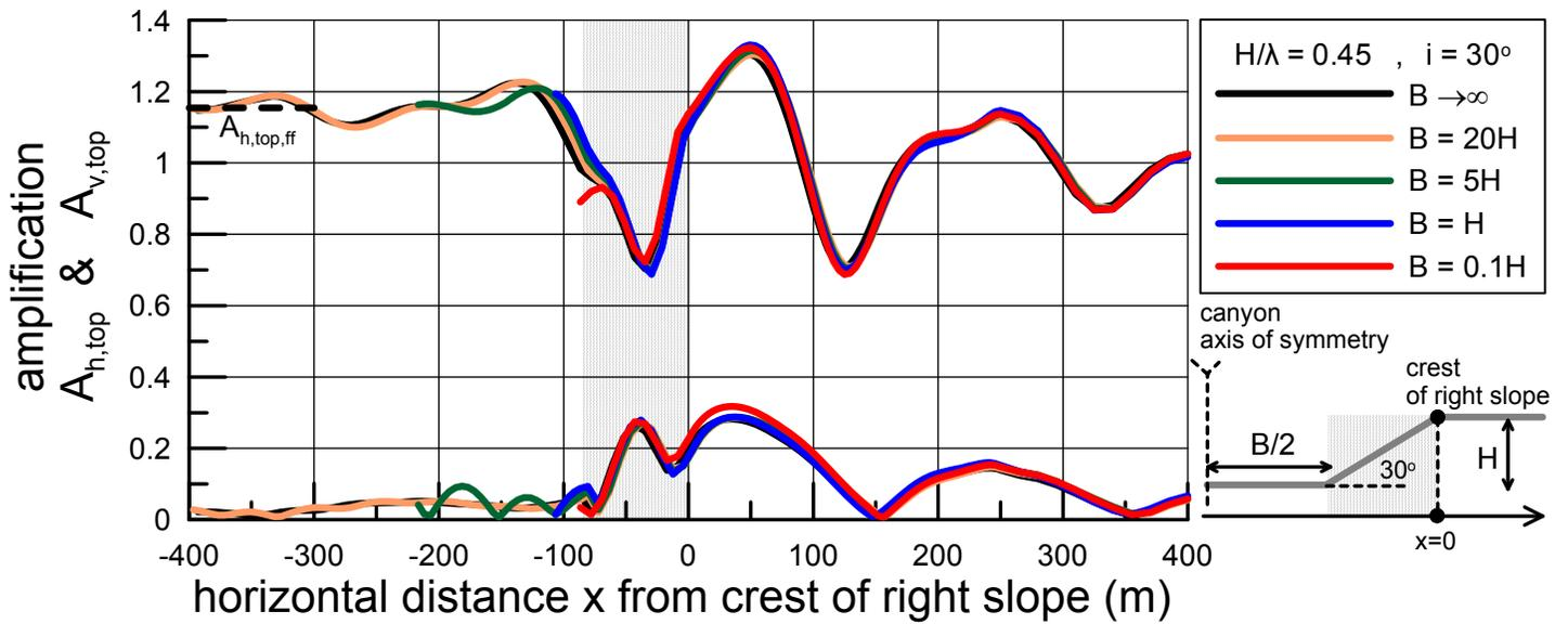
Fig. 4 Spatial variability of topographic aggravation factors  $A_{h,top}$  and  $A_{v,top}$  in the vicinity of symmetric trapezoidal canyons with slope inclination  $i=30^\circ$ , normalized height  $H/\lambda=0.45$  and various widths  $B = 0.1H, H, 5H, 20H$  and  $B \rightarrow \infty$ . Results are shown from the axis of symmetry of the canyon up to  $x=8H=400\text{m}$  behind the crest of the right slope.
