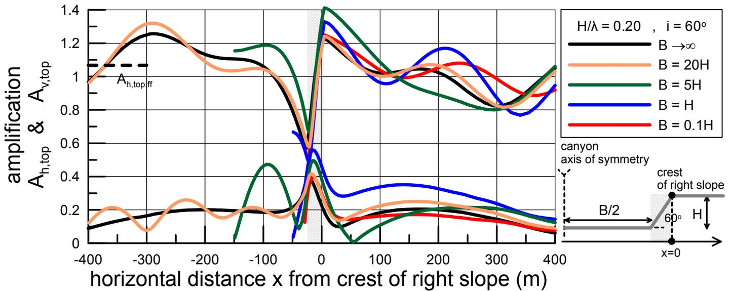
Fig. 7 Spatial variability of topographic aggravation factors  $A_{h,top}$  and  $A_{v,top}$  in the vicinity of symmetric trapezoidal canyons with slope inclination  $i=60^\circ$ , normalized height  $H/\lambda=0.20$  and various widths  $B = 0.1H, H, 5H, 20H$  and  $B \rightarrow \infty$ . Results are shown from the axis of symmetry of the canyon up to  $x=8H=400\text{m}$  behind the crest of the right slope.
