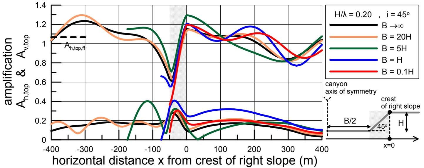
Fig. 5 Spatial variability of topographic aggravation factors  $A_{h,top}$  and  $A_{v,top}$  in the vicinity of symmetric trapezoidal canyons with slope inclination  $i=45^\circ$ , normalized height  $H/\lambda=0.20$  and various widths  $B = 0.1H, H, 5H, 20H$  and  $B \rightarrow \infty$ . Results are shown from the axis of symmetry of the canyon up to  $x=8H=400\text{m}$  behind the crest of the right slope.
