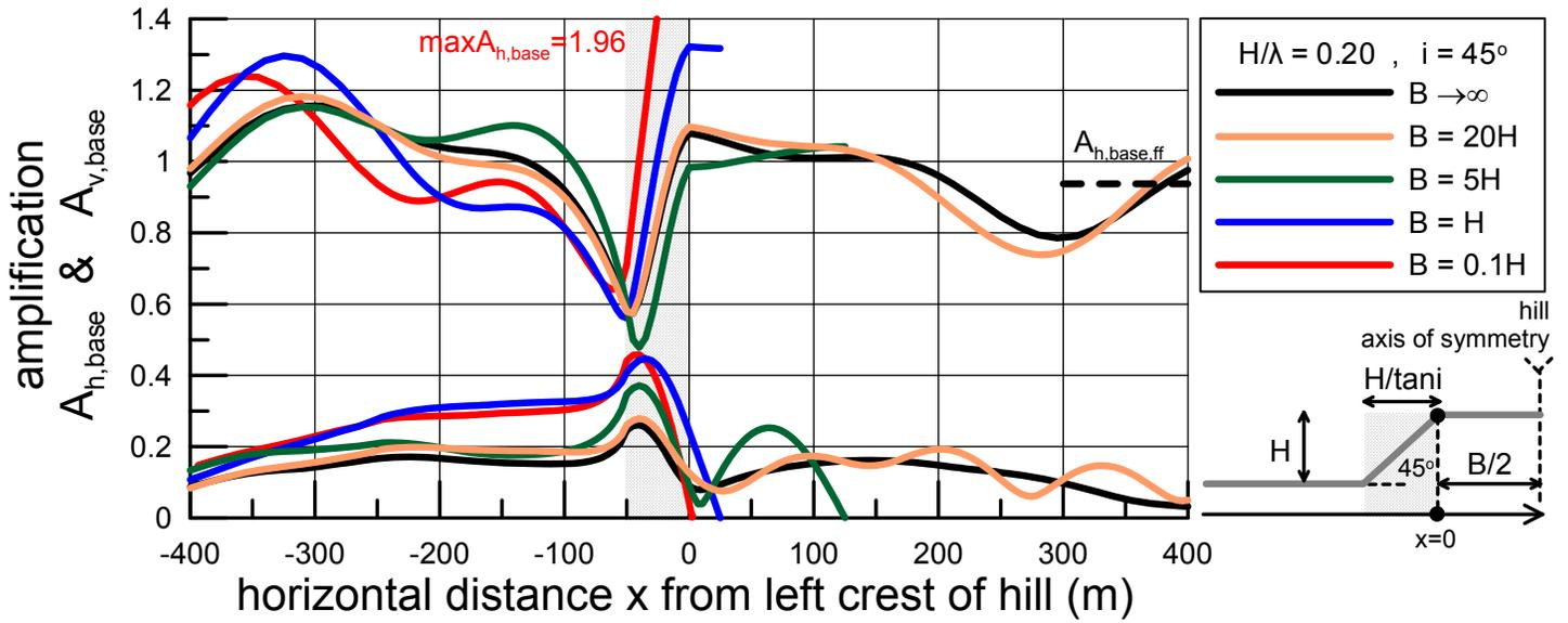
Fig. 11 Spatial variability of topographic aggravation factors  $A_{h,base}$  and  $A_{v,base}$  in the vicinity of symmetric trapezoidal hills with slope inclination  $i=45^\circ$ , normalized height  $H/\lambda=0.20$  and various widths  $B = 0.1H, H, 5H, 20H$  and  $B \rightarrow \infty$ . Results are shown from  $x=-8H=-400m$  in front of the toe of the left slope and reach the axis of symmetry of the hill.
