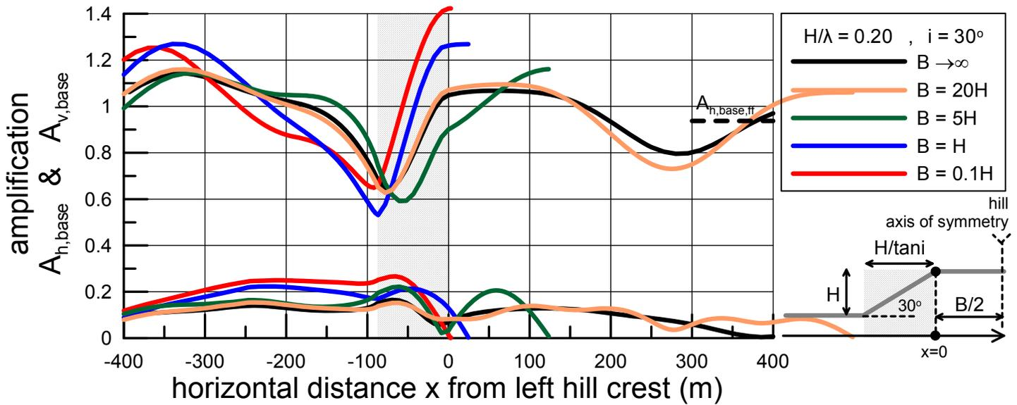
Fig. 9 Spatial variability of topographic aggravation factors  $A_{h,base}$  and  $A_{v,base}$  in the vicinity of symmetric trapezoidal hills with slope inclination  $i=30^\circ$ , normalized height  $H/\lambda=0.20$  and various widths  $B = 0.1H, H, 5H, 20H$  and  $B \rightarrow \infty$ . Results are shown from  $x=-8H=-400$ m in front of the toe of the left slope and reach the axis of symmetry of the hill.
