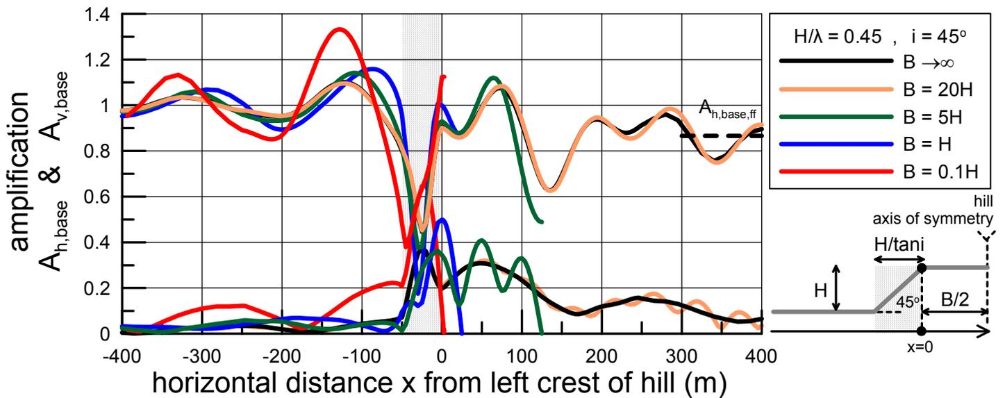
Fig. 12 Spatial variability of topographic aggravation factors  $A_{h,base}$  and  $A_{v,base}$  in the vicinity of symmetric trapezoidal hills with slope inclination  $i=45^\circ$ , normalized height  $H/\lambda=0.45$  and various widths  $B = 0.1H, H, 5H, 20H$  and  $B \rightarrow \infty$ . Results are shown from  $x=-8H=-400m$  in front of the toe of the left slope and reach the axis of symmetry of the hill.
