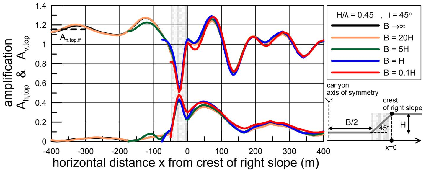
Fig. 6 Spatial variability of topographic aggravation factors  $A_{h,top}$  and  $A_{v,top}$  in the vicinity of symmetric trapezoidal canyons with slope inclination  $i=45^\circ$ , normalized height  $H/\lambda=0.45$  and various widths  $B = 0.1H, H, 5H, 20H$  and  $B \rightarrow \infty$ . Results are shown from the axis of symmetry of the canyon up to  $x=8H=400\text{m}$  behind the crest of the right slope.
