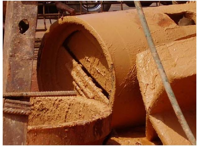
Fig.8 Close up view of chisel and bailer
