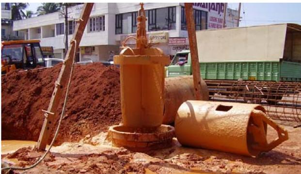
Fig. 7 Chisel and bailer for bored piles
