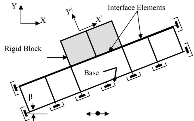
Fig. 14. Finite difference model (only FLAC<sup>TM</sup> macro elements shown) of an inclined base shaking table test (Arab et al. 2010).
