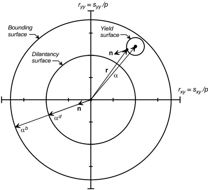
Fig. 3. Schematic of the bounding, dilation, and yield surfaces on the  $r_{yy}$ - $r_{xy}$  stress-ratio plane with the yield surface, normal tensor, dilatancy back stress ratio, and bounding back stress ratio.
