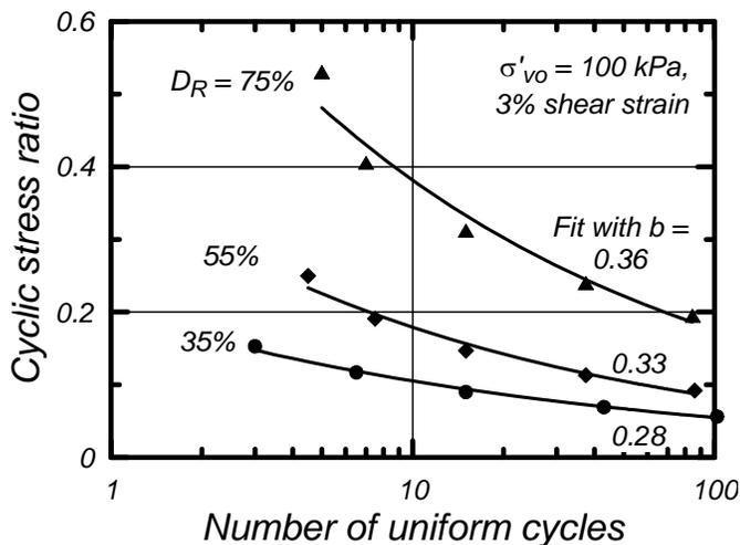
Fig. 6. Cyclic stress ratios versus number of uniform loading cycles in undrained DSS loading to cause single-amplitude shear strains of 3% for  $D_R = 35, 55,$  and  $75\%$  with a vertical effective consolidation stress of 1 atm. Each set of CSR-N simulations was fit with a power relationship and the exponent  $b$  labeled beside each curve
