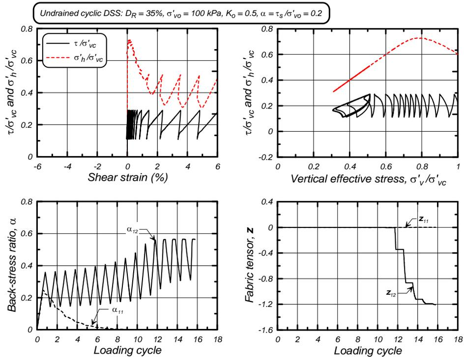
Fig. 5. Undrained cyclic DSS loading response for  $D_R = 35\%$  with an initial static shear stress ratio of 0.2, showing the variation in stresses, strains, back-stress ratios, and fabric tensor terms.
