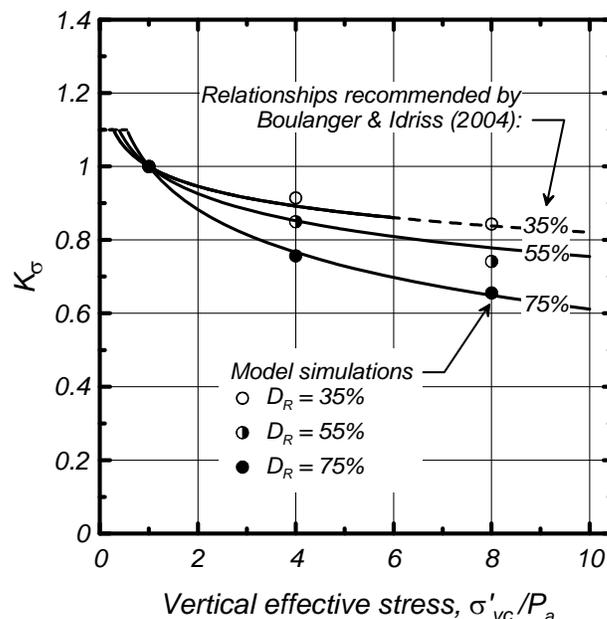
Fig. 7. Comparison of  $K_\sigma$  factors from simulations versus relationships by Boulanger and Idriss (2004).
