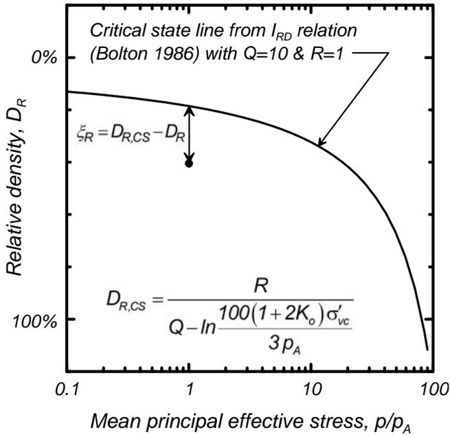
Fig. 1. Definition of the relative state parameter index,  $\xi_R$  (Boulanger 2003) and the effects of varying  $Q$  and  $R$
