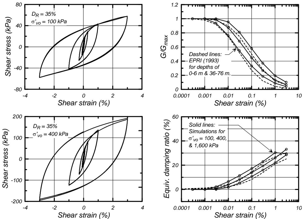
Fig. 8. Drained strain-controlled cyclic DSS loading responses for  $D_R = 35\%$  under vertical effective consolidation stresses of 1, 4, and 16 atm.
