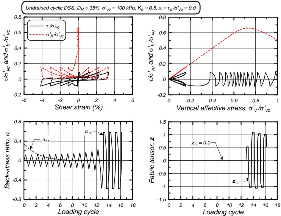
Fig. 4. Undrained cyclic DSS loading response for  $D_R = 35\%$  with an initial static shear stress ratio of 0.0, showing the variation in stresses, strains, back-stress ratios, and fabric tensor terms.
