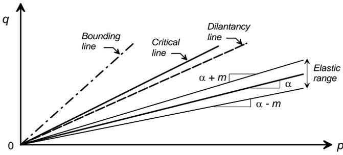
Fig. 2. Schematic of yield, critical, dilatancy, and bounding lines in  $q$ - $p$  space (after Dafalias & Manzari 2004)
