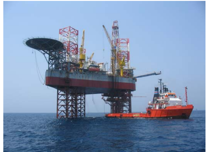
Fig. 1. Jack-ups are large, self elevating platforms used to drill offshore oil and gas wells.
