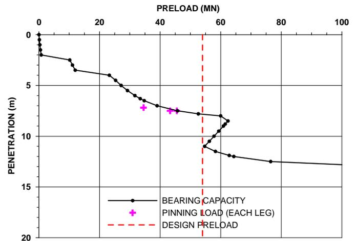
Fig. 4. Example of prediction of leg penetration curve.
