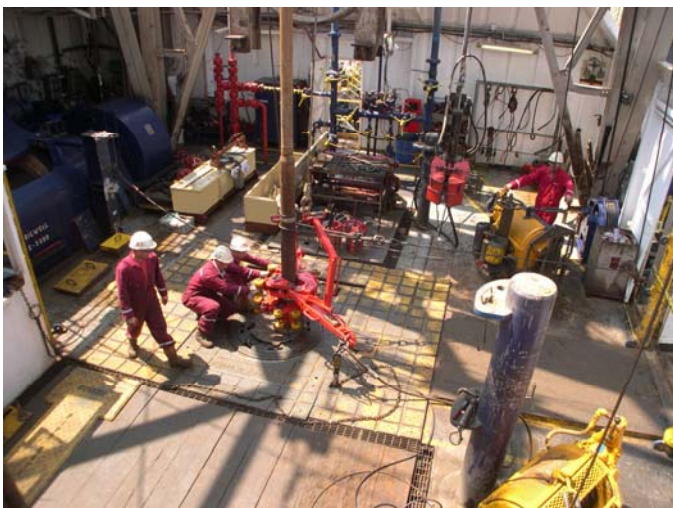
Fig. 3. A view of the drill floor of a jack-up rig during building of the drill strings, previous to start sampling.
