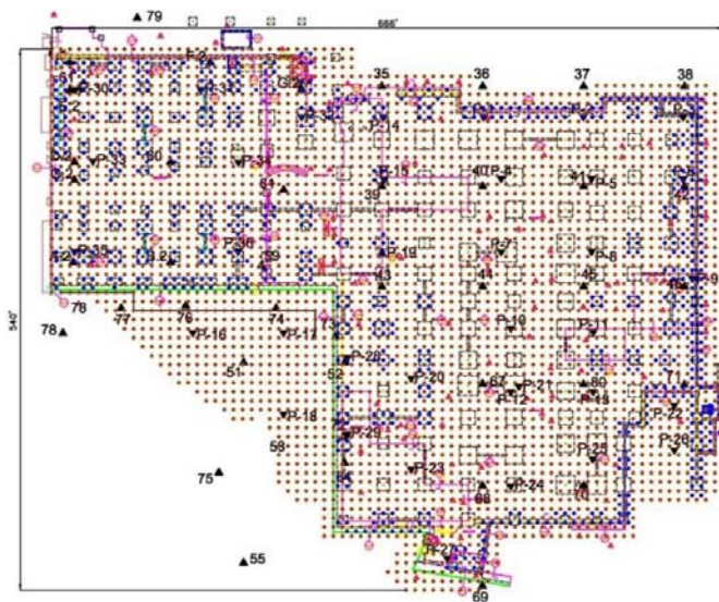
Fig 3. Stone column layout, the red and blue dots show the primary and secondary columns.
