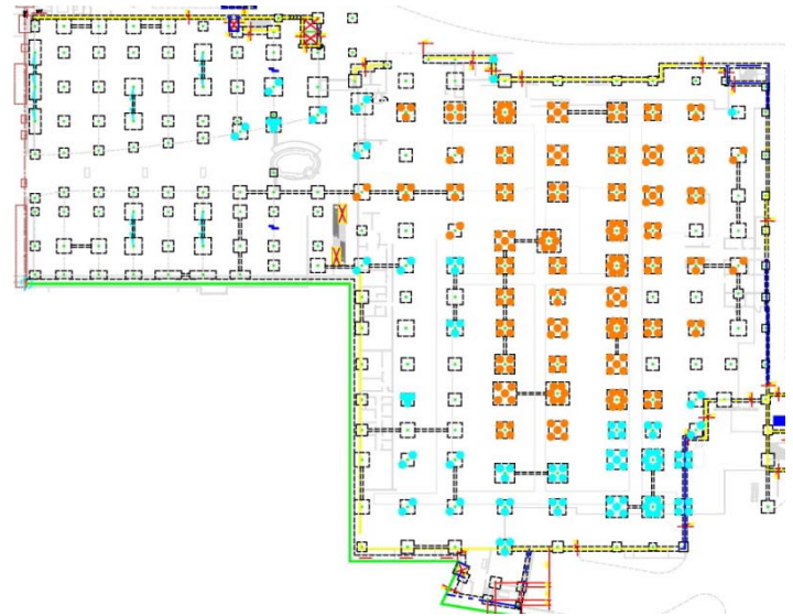
Fig 4. Soil mix columns under heavily loaded footings. Blue dots = 25 ft (7.6) and brown dots = 35 ft (10.6 m) columns.
