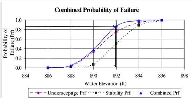
Figure 11 Waterworks Unit, Combined Probability of Failure
