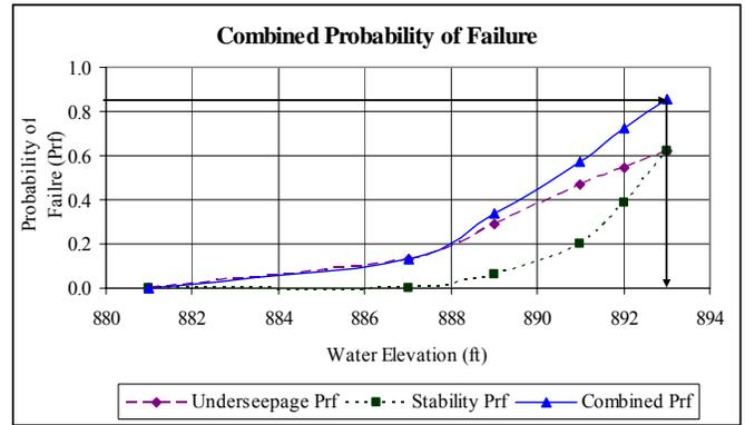
Figure 12 South Topeka Unit, Combined Probability of Failure
