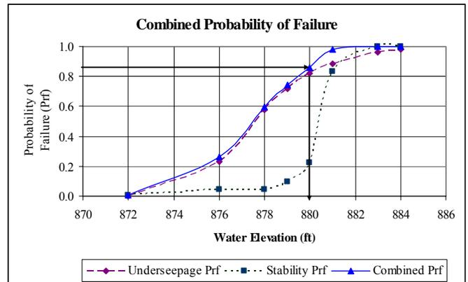
Figure 13 Oakland Levee Unit Combined Probability of Failure
