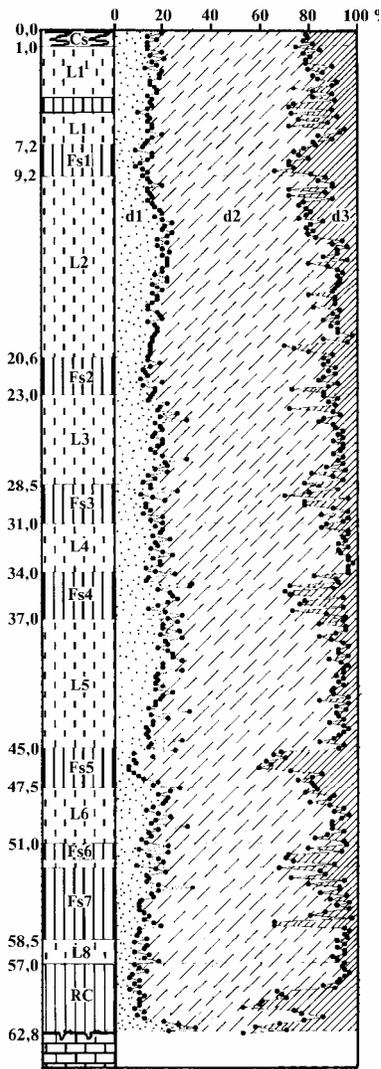
Fig. 2. Typical changes in the grain-size distribution of loess with depth (borehole near the Lyubenovo village, Svishtov district).
