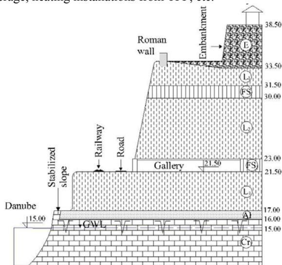
Fig. 5. Underground gallery in Rousse with an entrance in the slope base; L – loess; FS – fossil soil; Al – alluvium of gravels and sands; Cr<sub>1</sub> – Lower Cretaceous limestones.
