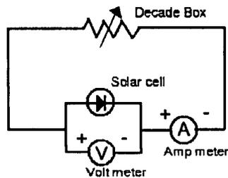
Fig. 3.2. Circuit for measuring solar cell characteristic
