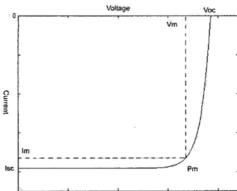
Fig. 2.3. Characteristic curve of the solar cell
