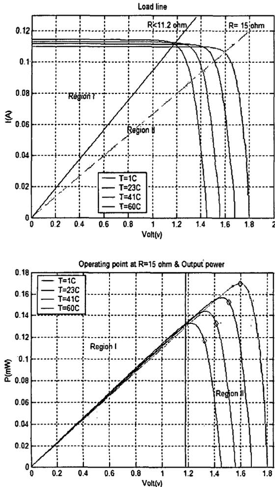
Fig. 4.4. Two loading regions and corresponding power curves
