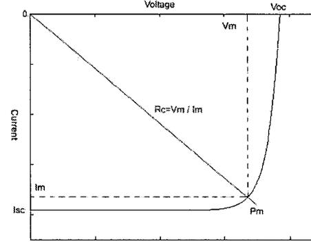
Fig. 2.4. Characteristic resistance load line
