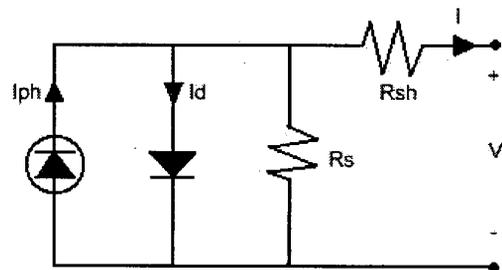
Fig. 2.2 Equivalent circuit of the solar cell
