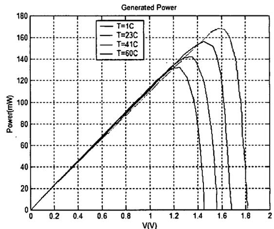
Fig. 3.4. Power output as a Function of Temperature
