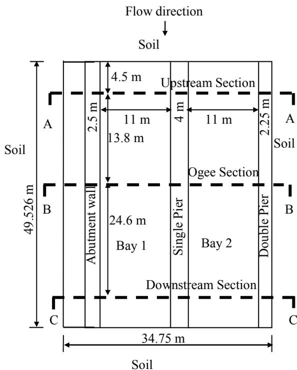
Fig. 1. Plan showing various comparative sections of bays 1-2
