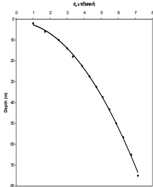
Fig. 3. Parabolic variation of modulus of elasticity ( $E_s$ ) with depth for non-homogeneous soil medium
