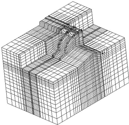
Fig. 5. 3D-Finite element model of bays 1-2 with pier, raft and foundation soil
