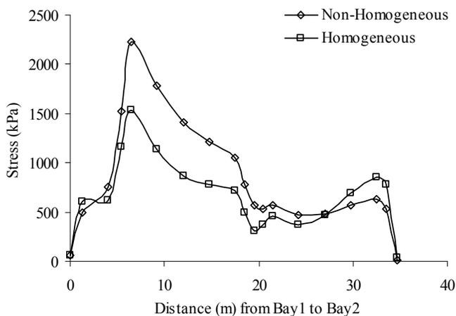
Fig. 9. Comparative stress at downstream section (C-C)
