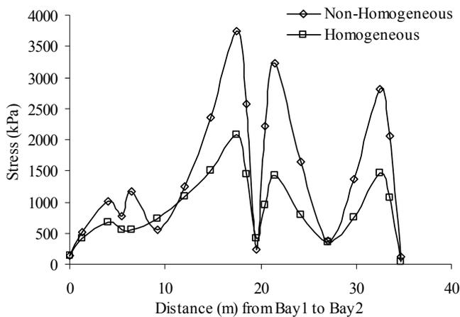
Fig. 8. Comparative stress at ogee section (B-B)
