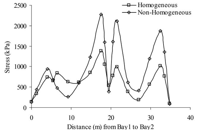
Fig. 7. Comparative stress at upstream section (A-A)
