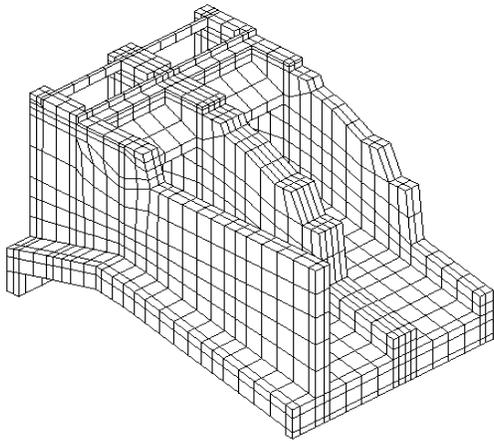
Fig. 4. 3D-Finite element discretization of the pier, abutment and raft system with cut-off of bays 1-2
