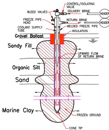
Fig.2 Typical Details of a Freeze Pipe
