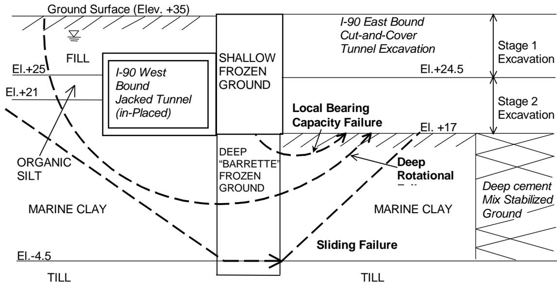
Fig.8 Typical Cross Section with the Proposed Excavation Stages and Various Stability Failure Modes
