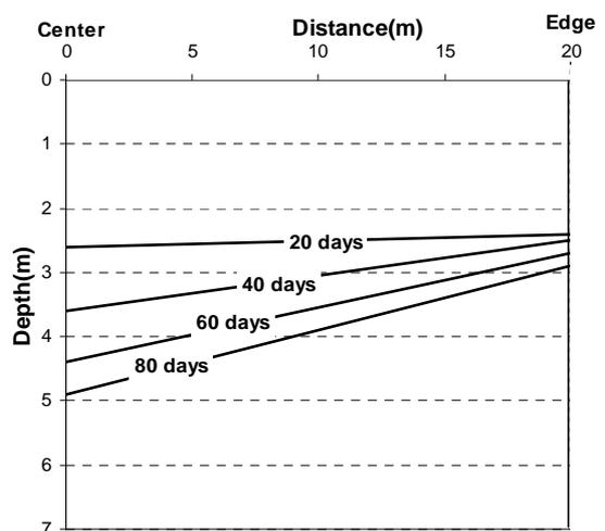
Figure 8. Change in position of zero value pore pressure line
