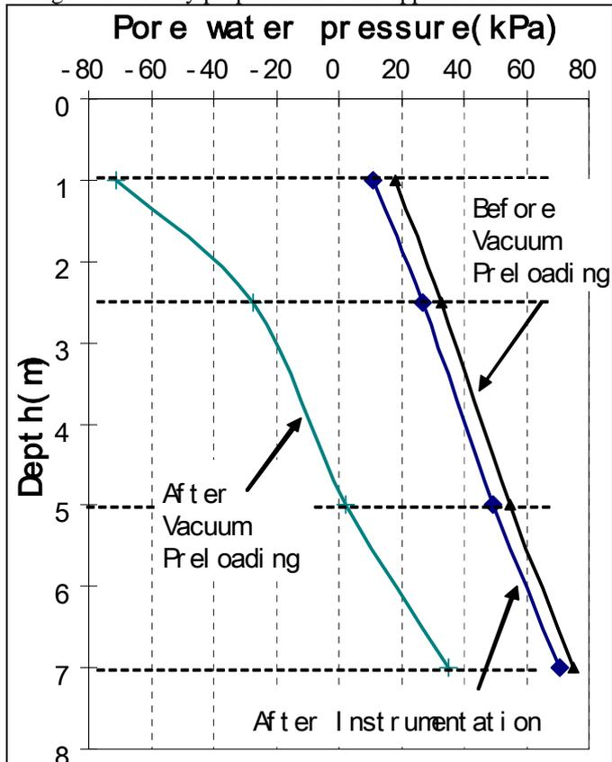
Figure 6. Variation of pore water pressures with depth
