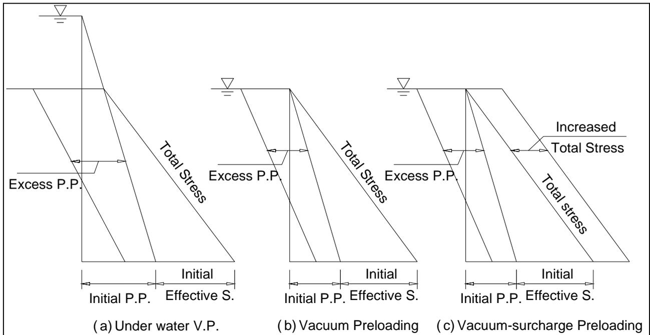
Figure 9. Comparison of mechanism of different vacuum methods
