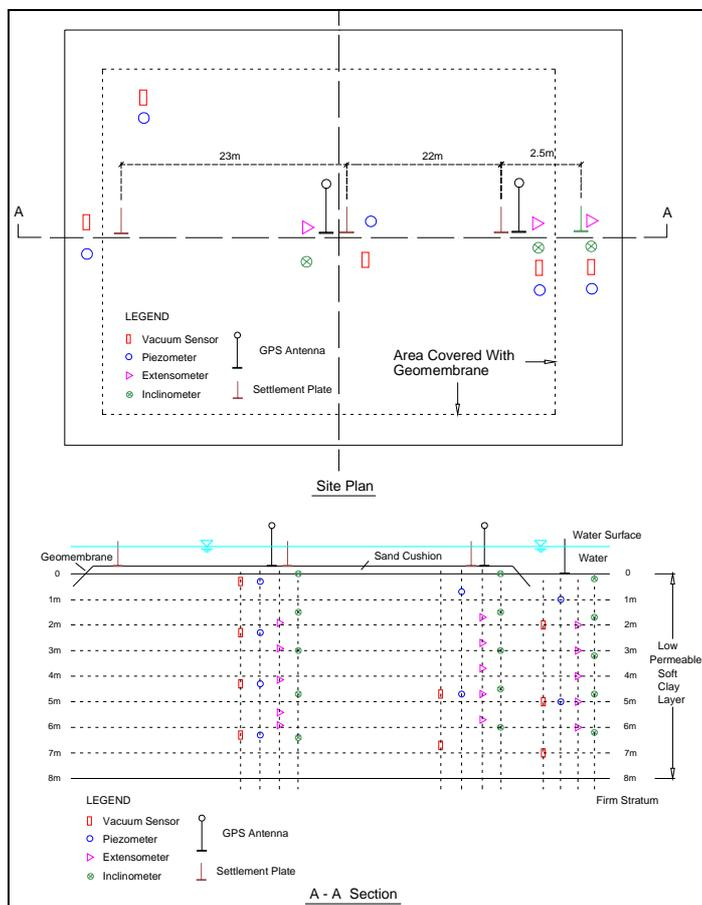
Figure 3. Layout and cross-section view of instrumentation
