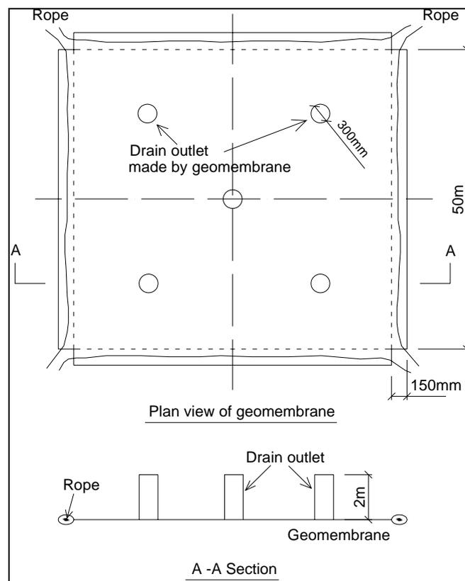
Figure 2. Schematic diagram of custom made geomembrane
