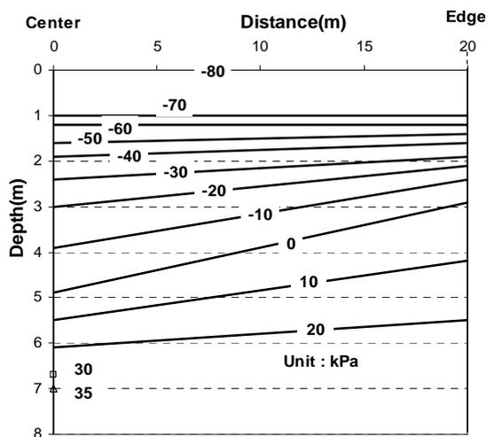
Figure 7. Contour of excess pore pressure after 80 days
