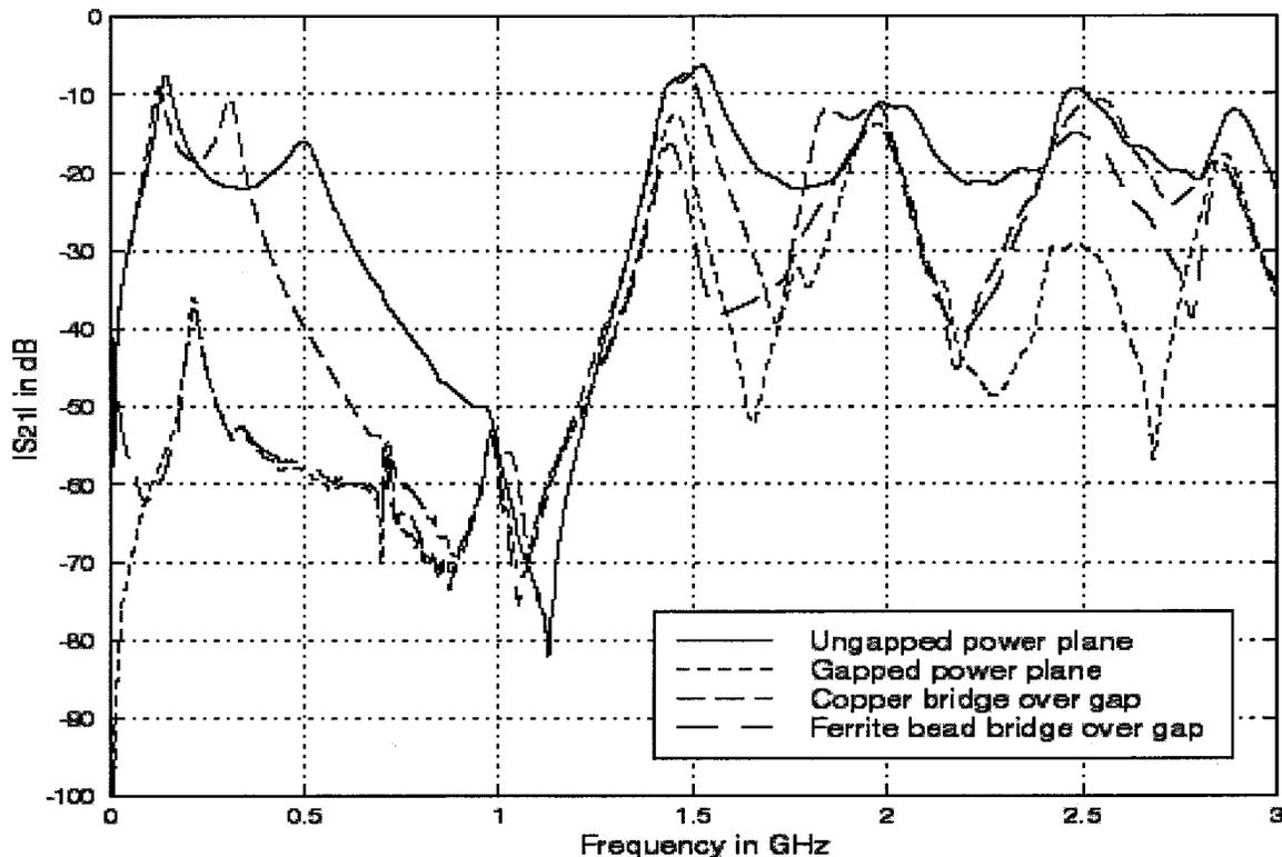
Fig. 7. Effect of connections bridging the power islands.
