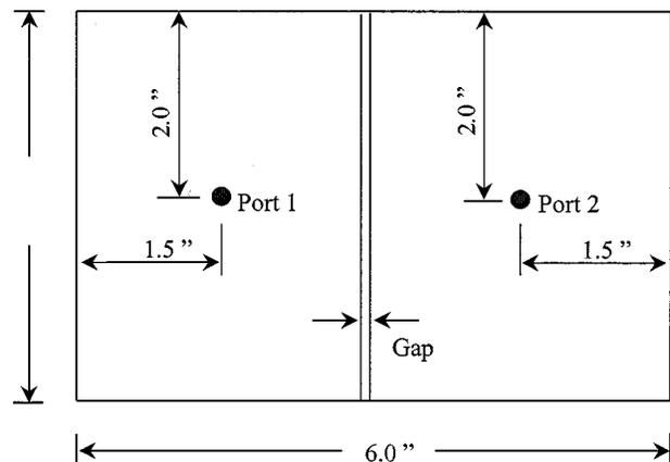
Fig. 1. Layout of boards 1 and 2.
