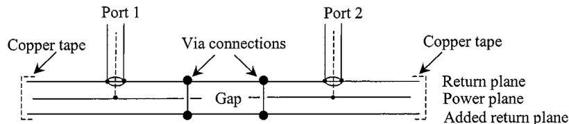
Fig. 8. Three-layer board stack-up.
