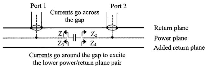
Fig. 10. Current path in the three-layer board.
