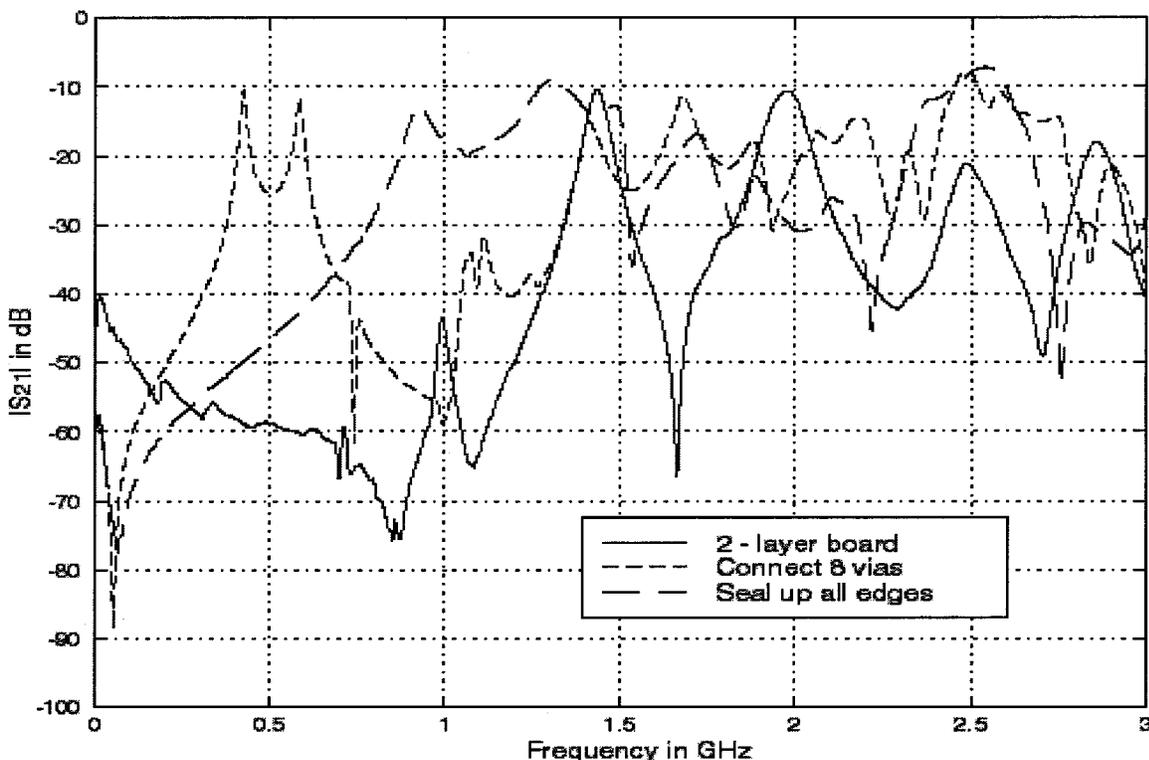
Fig. 9.  $|S_{21}|$  for two-layer and three-layer boards.
