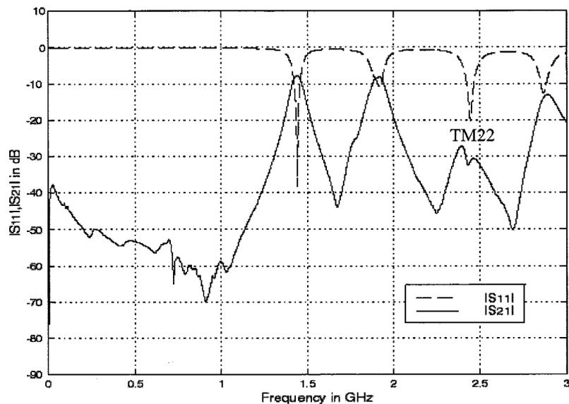
Fig. 6. Measured  $|S_{11}|$  and  $|S_{22}|$  for board 1.
