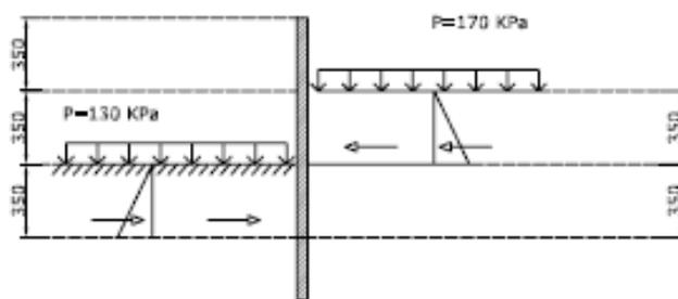
Fig. 9. The schema for calculation of second phases.
