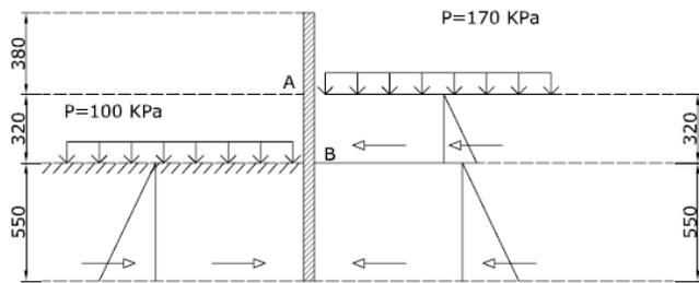
Fig.6. Verification of sheet pile walls after putting 4m concrete on the bottom of hole ( $\Sigma Er = 1132 \text{ KN/m}$ ;  $\Sigma EI = 1830 \text{ KN/m}$ ).
