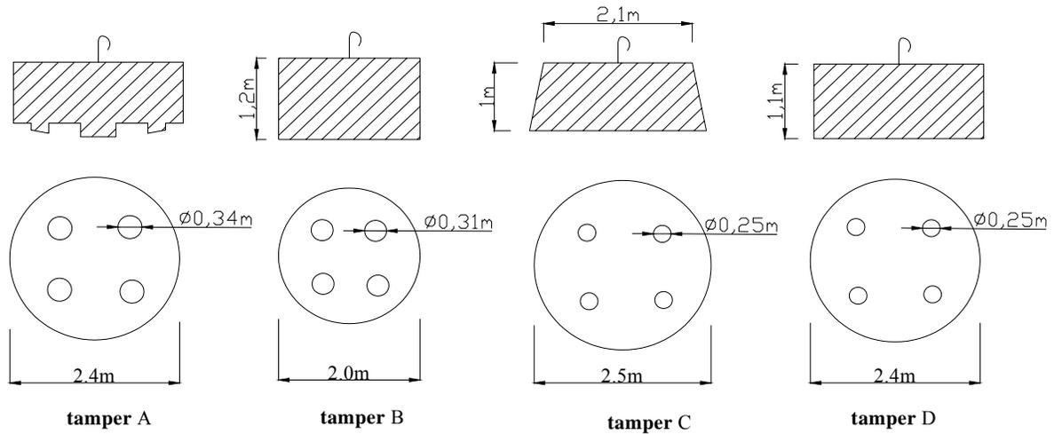
Fig. 2 Geometry characteristic of the tampers
