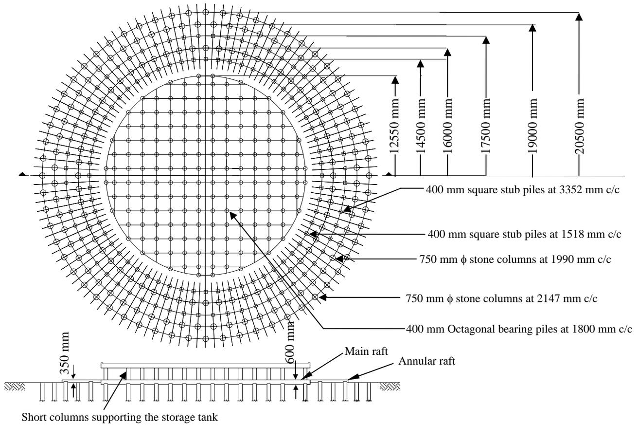
Fig. 3 Foundation system for phosphoric acid storage tank
