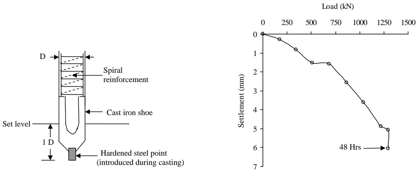
Fig.4 Details of pile toe
